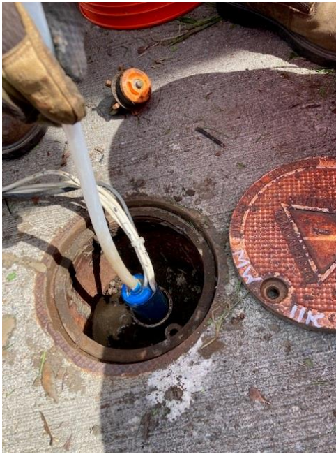
MW-11K showing depth at which Whale Pump could not descend further.
