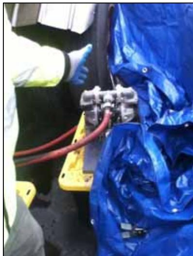
Double diaphragm chemical resistant pump located in the secondary containment next to the air compressor. The blue tarp was used to keep the pump and air supply warm during sub-freezing conditions.
