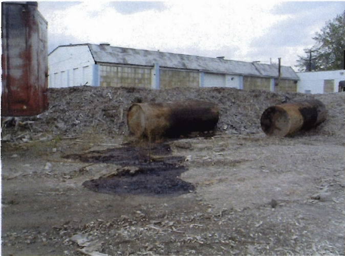
Photograph No. 5 - Two large tanks and an associated area of staining were observed at the Raeco site in September 1999. Surface soil sample SS-2 was collected from this area of staining on November 10, 1999, after the tanks had been removed.
