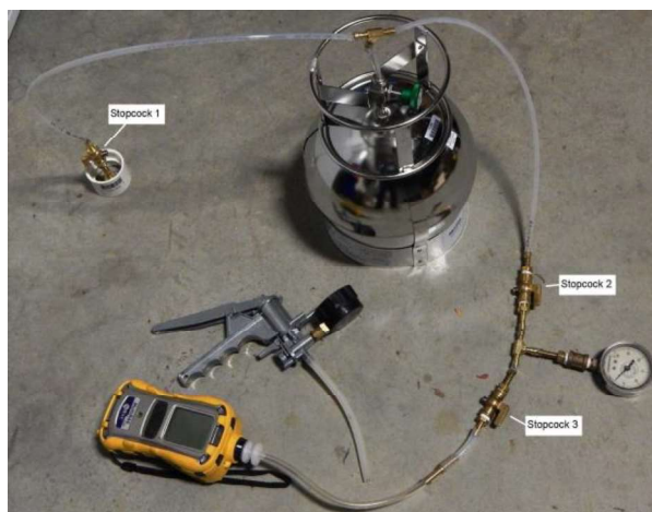
Figure 1. Example of Sub-Slab Sampling and Leak-Test Setup
