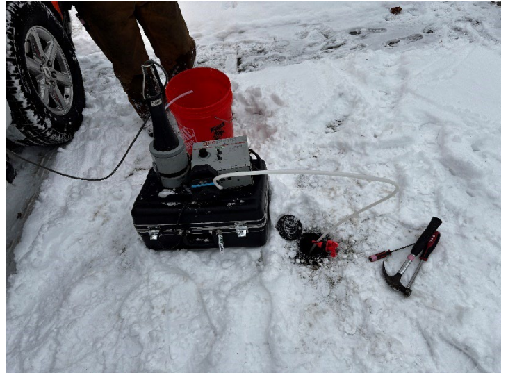
Groundwater purge setup on DP-20
