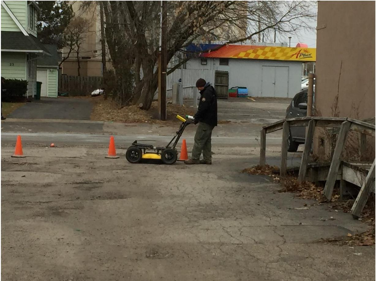
Photo #4: Thew Associates using a Ground Penetrating Radar to determine the location of buried features.
