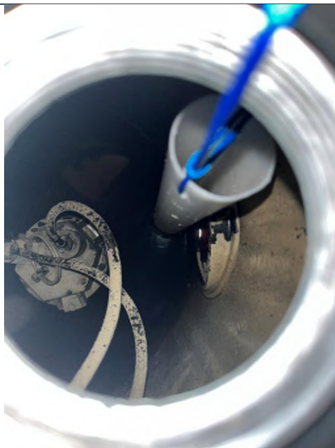
Bailer with thiosulfate crystals for neutralization.
