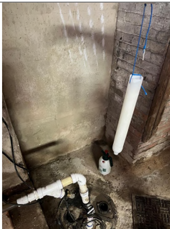
Bailer with thiosulfate crystals for neutralization.
