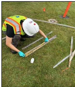
Photo 3: Image of Pre-Injection Cores being sampled.
