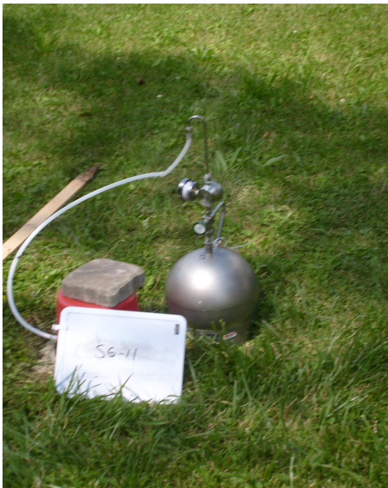
Photo 12: Soil vapor sampling with helium enclosure at SG-11.
