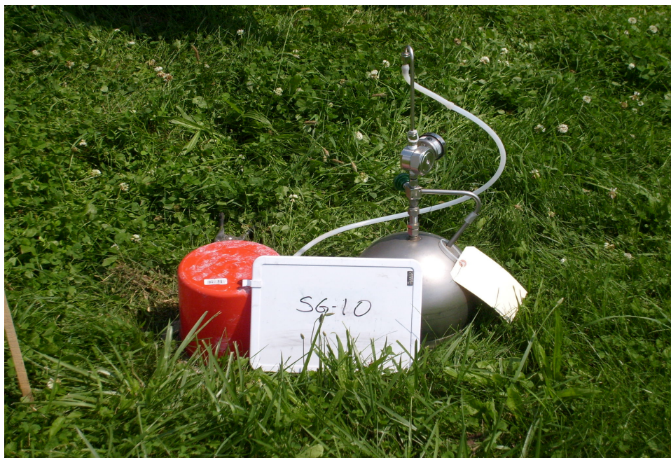
Photo 11: Soil vapor sampling with helium enclosure at SG-10.
