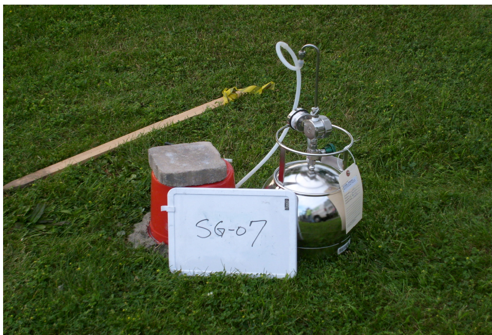
Photo 8: Soil vapor sampling with helium enclosure at SG-07.
