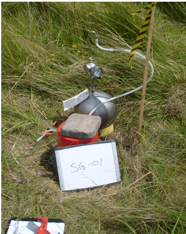
Photo 2: Soil vapor sampling with helium enclosure at SG-01.
