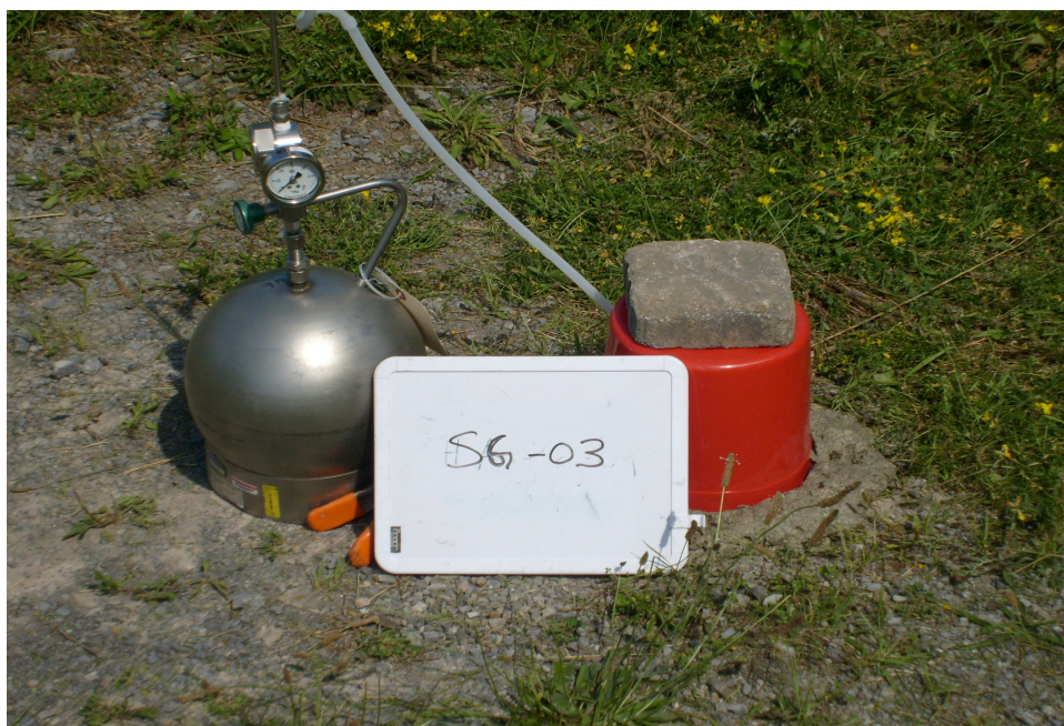
Photo 4: Soil vapor sampling with helium enclosure at SG-03.
