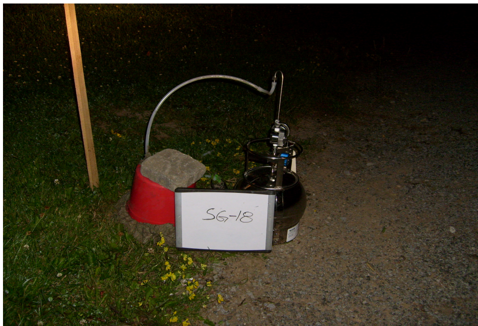
Photo 19: Soil vapor sampling with helium enclosure at SG-18.
