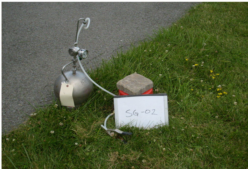
Photo 3: Soil vapor sampling with helium enclosure at SG-02.
