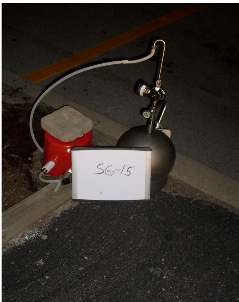
Photo 16: Soil vapor sampling with helium enclosure at SG-15.
