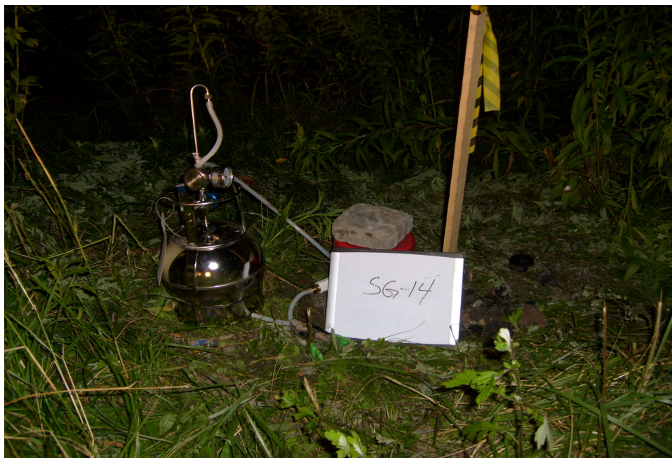
Photo 15: Soil vapor sampling with helium enclosure at SG-14.
