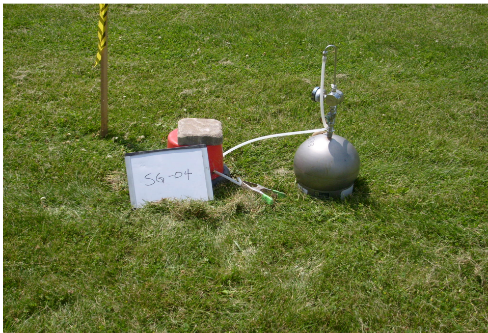
Photo 5: Soil vapor sampling with helium enclosure at SG-04.
