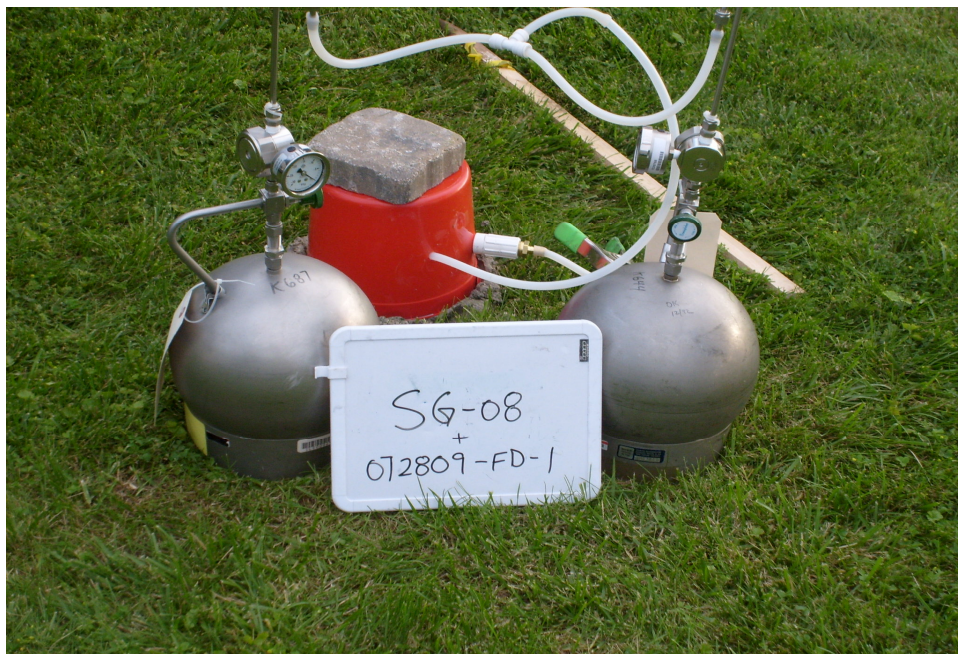
Photo 9: Soil vapor sampling with helium enclosure at SG-07 and field duplicate 072809-FD-1
