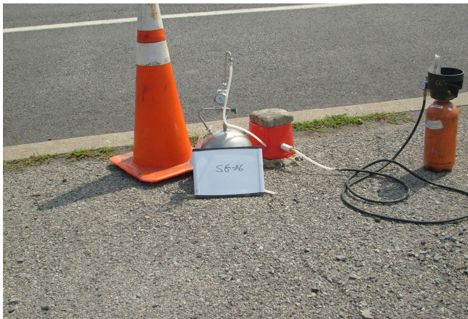
Photo 7: Soil vapor sampling with helium enclosure at SG-06.
