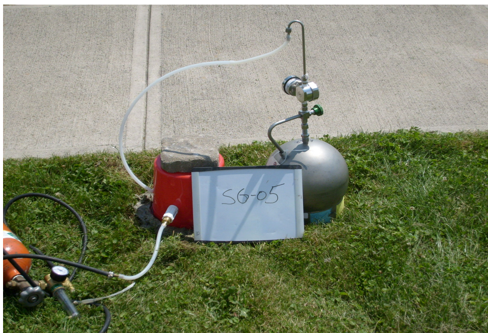
Photo 6: Soil vapor sampling with helium enclosure at SG-05.
