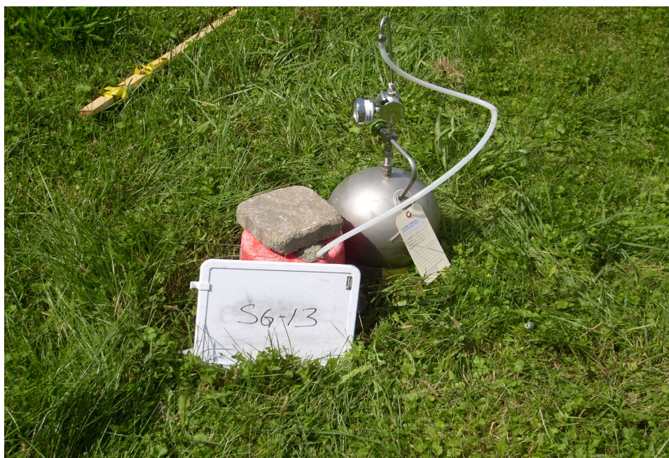
Photo 14: Soil vapor sampling with helium enclosure at SG-13.
