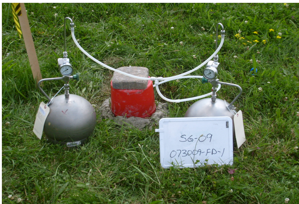
Photo 10: Soil vapor sampling with helium enclosure at SG-09 and field duplicate 073009-FD-1.
