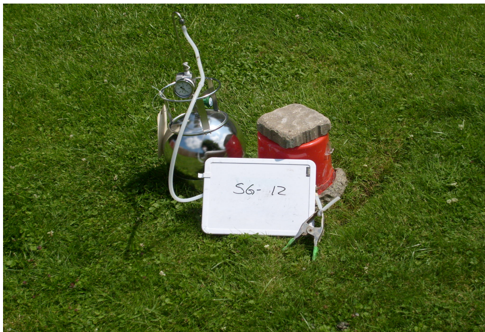
Photo 13: Soil vapor sampling with helium enclosure at SG-12.
