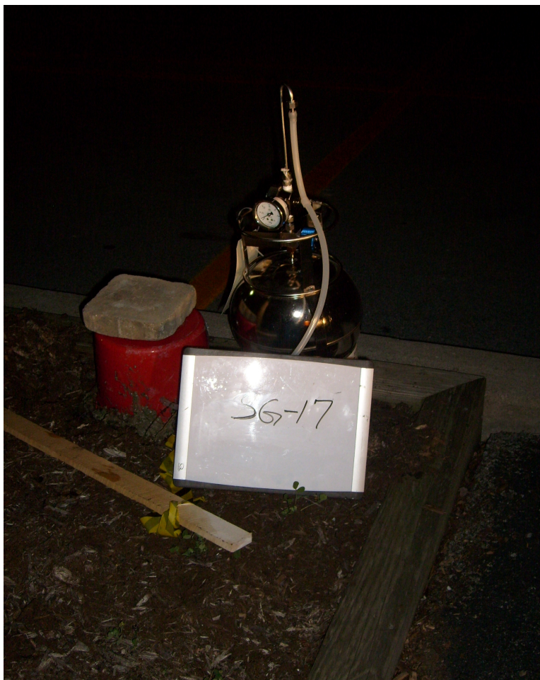
Photo 18: Soil vapor sampling with helium enclosure at SG-17.
