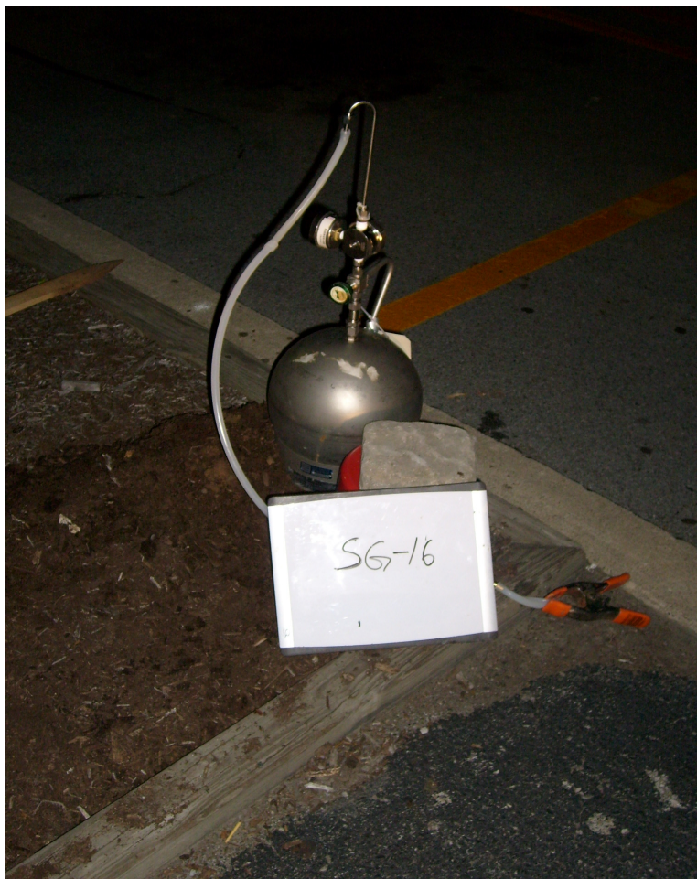
Photo 17: Soil vapor sampling with helium enclosure at SG-16.
