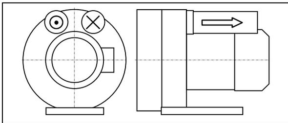
Fig. 4: 2BH1840-7G... (two-impeller pump-motor unit with double-flow design)
