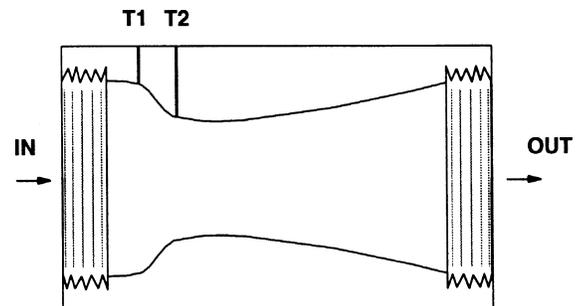
Rotron's flow meter is a venturi style design. After air enters the inlet, the pressure is measured in the T1 tap. The second tap, T2, measures the pressure at the throat. The differential between T1 and T2 registers across a special calibrated CFM gauge to provide accurate readings. The throat is then expanded back to the original size to keep pressure loss to under 2-4 IWG.
