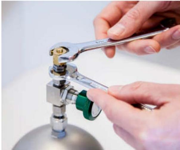
**Photo 3: Top of Summa Canister, Removing Cap**
