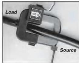
**IMPORTANT:** When looking from the source side of the conductor(s) being monitored, you should see the arrow on the current sensor assembly. The arrow should be pointing in a clockwise direction around the conductor(s) being monitored. If the arrow is not positioned on the source side, inaccurate readings will result.
