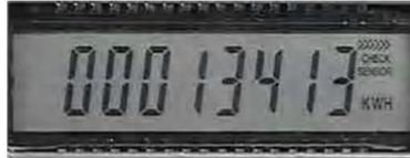
The Class 2000 kWh meter display requires no multiplier and shows kilowatt-hours consumed. See section 6.2 for information on calculating cost based on kWh usage.
