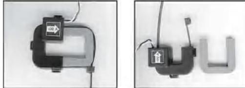
STEP 2: Reassemble the current sensor assembly around the conductor(s) to be monitored. Ensure the current sensor halves marked "Load" are both facing the load side of the conductor. The colored arrow will be on the source side of the conductor being monitored and MUST be pointed in a clockwise direction around the conductor being monitored. Tighten the nylon clamp to complete the assembly.
