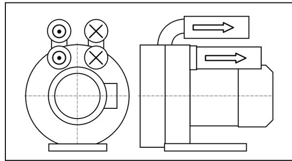
Fig. 6: 2BH1840-7L... (two-impeller pump-motor unit with double-flow design)
