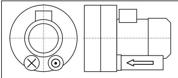
Fig. 3: 2BH1640 (two-impeller pump-motor unit with double-flow design)
