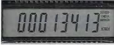
The Class 2000 kWh meter displays readings in whole numbers, there are no decimals.
