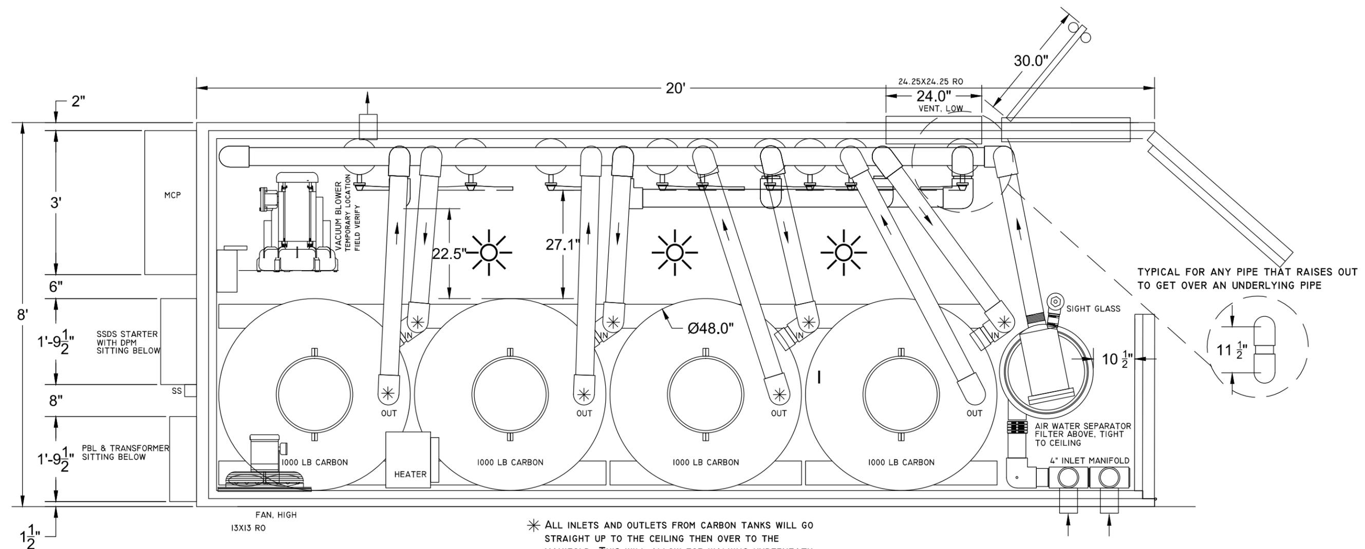
\* ALL INLETS AND OUTLETS FROM CARBON TANKS WILL GO STRAIGHT UP TO THE CEILING THEN OVER TO THE MANIFOLD. THIS WILL ALLOW FOR WALKING UNDERNEATH. FIELD VERIFY THE HEIGHT UP AND THE ANGLE OVER TO THE MANIFOLD.
