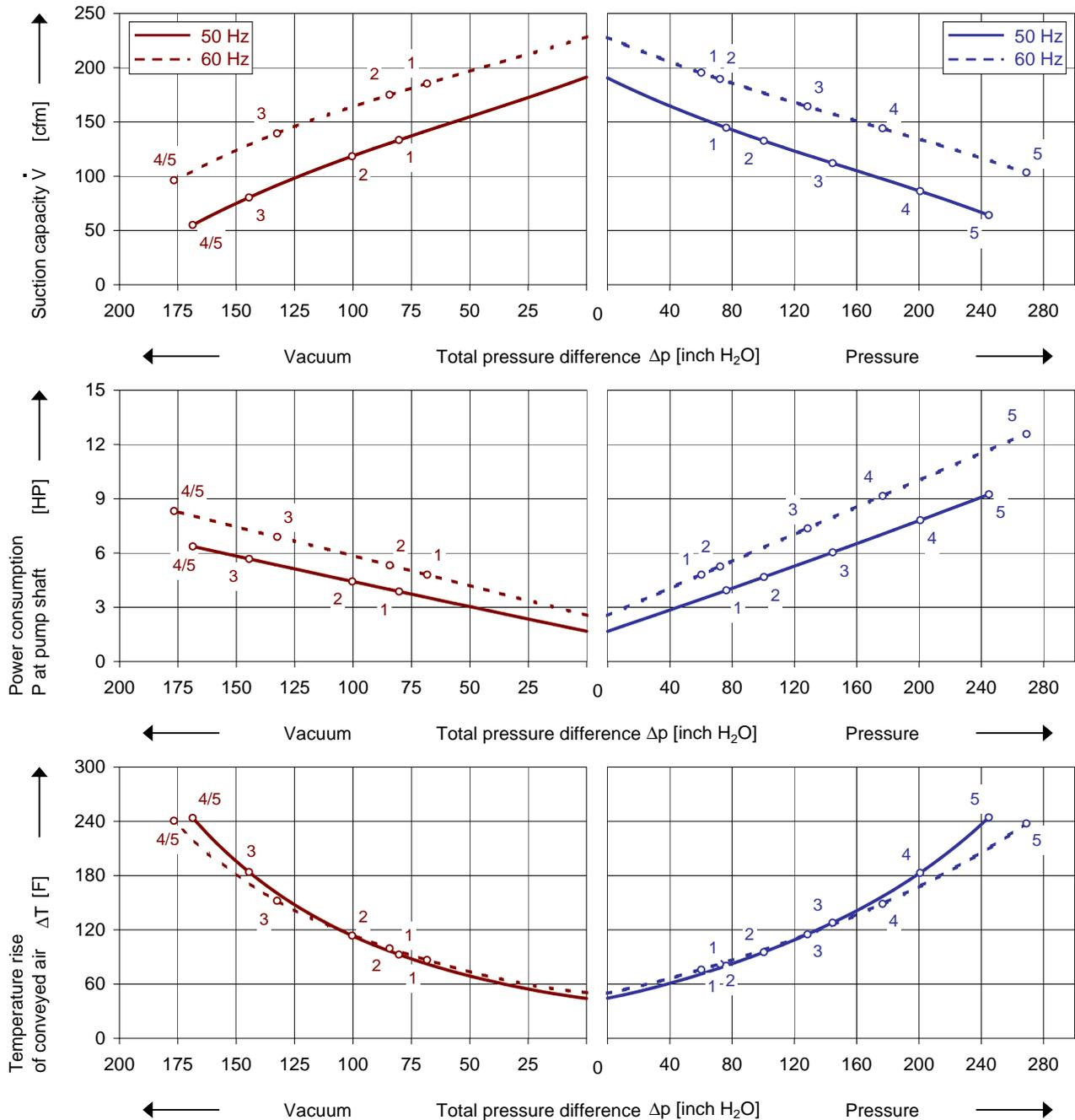
The performance curves are based on air at a temperature of 59 F and an atmospheric pressure of 29.91 inch Hg with a tolerance of ± 10 %. The total pressure differences are valid for inlet and ambient temperature up to 77 F. Suction capacity relates to inlet conditions. Pressure capacity relates to atmospheric conditions. For other conditions please get in touch with us.
