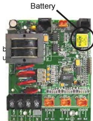
The battery cell is mounted in a socket on the right side of the main power board. Should the battery drop below 2.4 VDC in capacity, the display will illuminate a battery symbol on the left margin indicating a low condition. Additionally, the internal firmware will set a flag indicating the low battery condition. Use the following procedure to replace the lithium battery cell.
