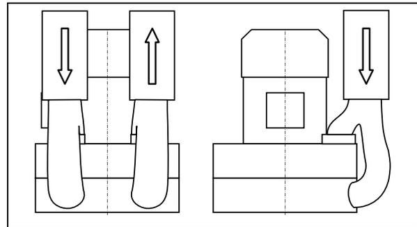
Fig. 7: 2BH1943 (two-impeller pump-motor unit with double-flow design)
