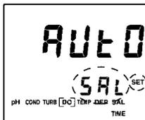
3. From the screen on which the value is displayed, use the **UP/DOWN** (**▲ ▼**) keys to enter the setting value if the salinity is known.
