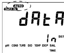
4. Press the **SET** key to display the screen for setting the data storage interval (A).
