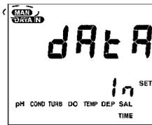
4. Press the **MEAS** key to return to the Measurement mode.
