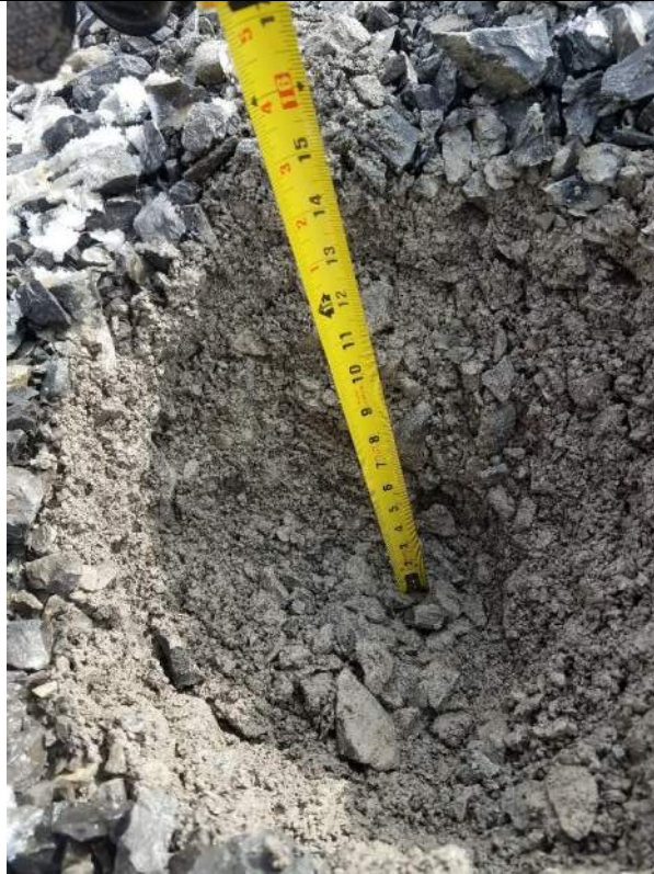
RAOC 3 El. 6 – Cover thickness at 12"
