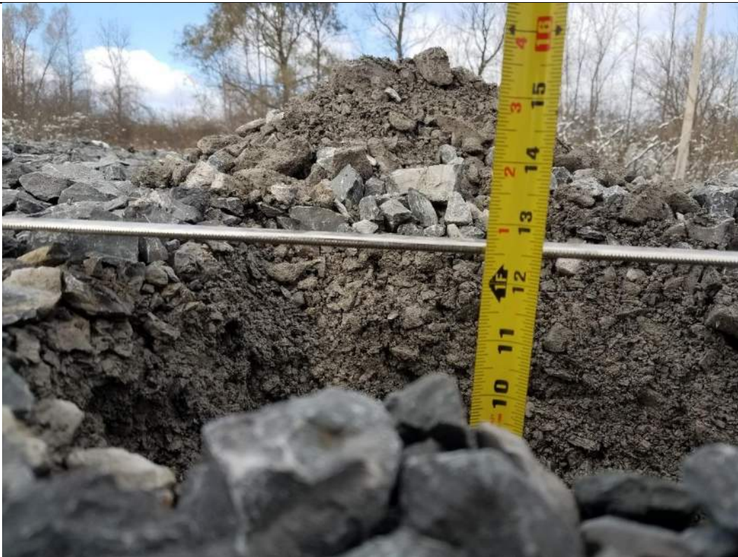
RAOC 3 El. 9 – Cover thickness at 12.5"
