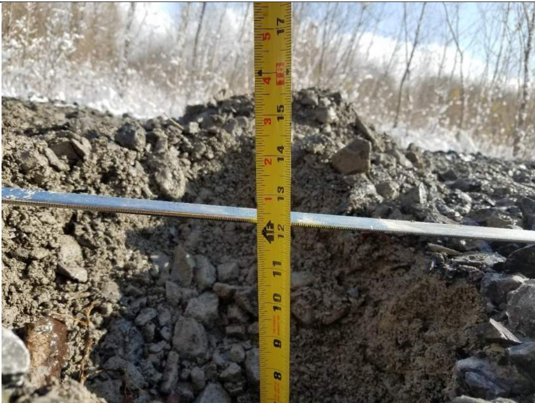
RAOC 3 El. 7 – Cover thickness at 12"
