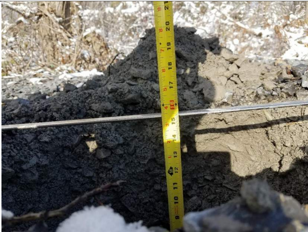
RAOC 3 El. 8 – Cover thickness at 15.5"
