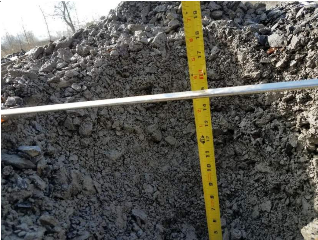
RAOC 3 El. 13 – Cover thickness at >15.5"
