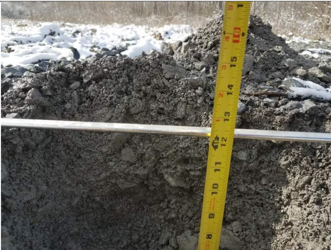
RAOC 3 El. 13 – Cover thickness at 12.25"
