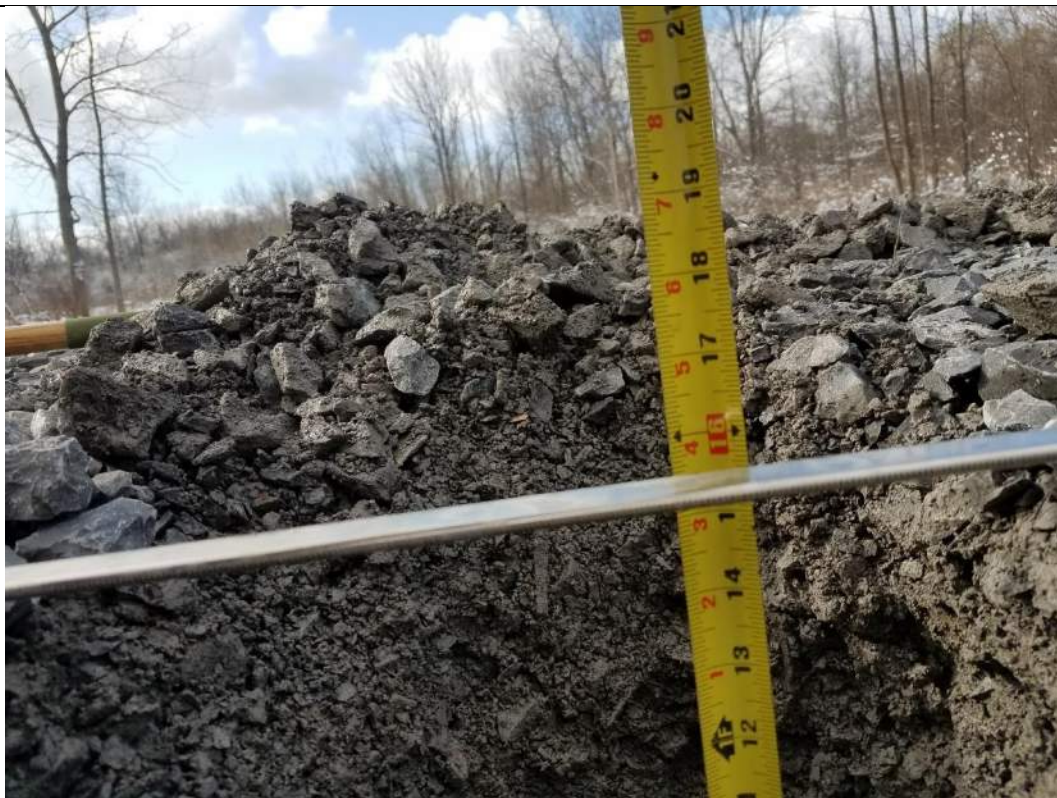
RAOC 3 El. 11 – Cover thickness at 15.75"
