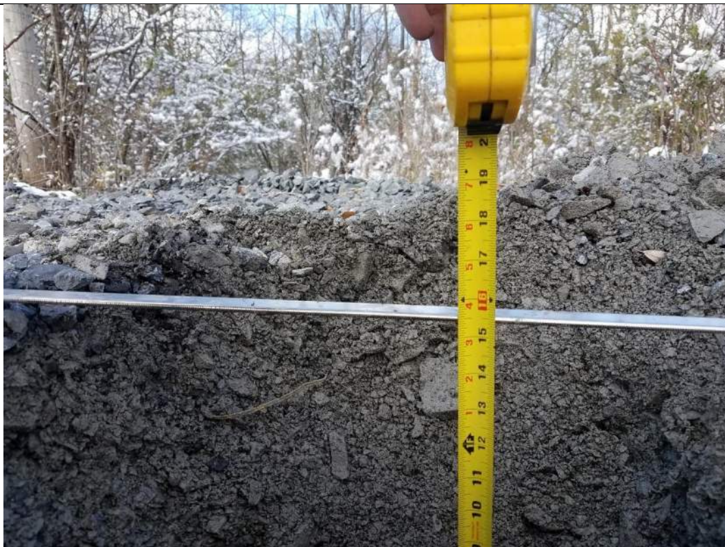
RAOC 3 El. 12 – Cover thickness at >15.75"
