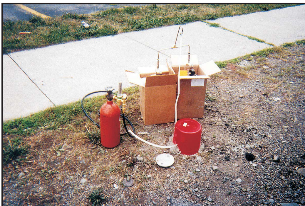
Photo 27: Photograph looking south at tracer gas and summa canister set-up at SG-10 location.
