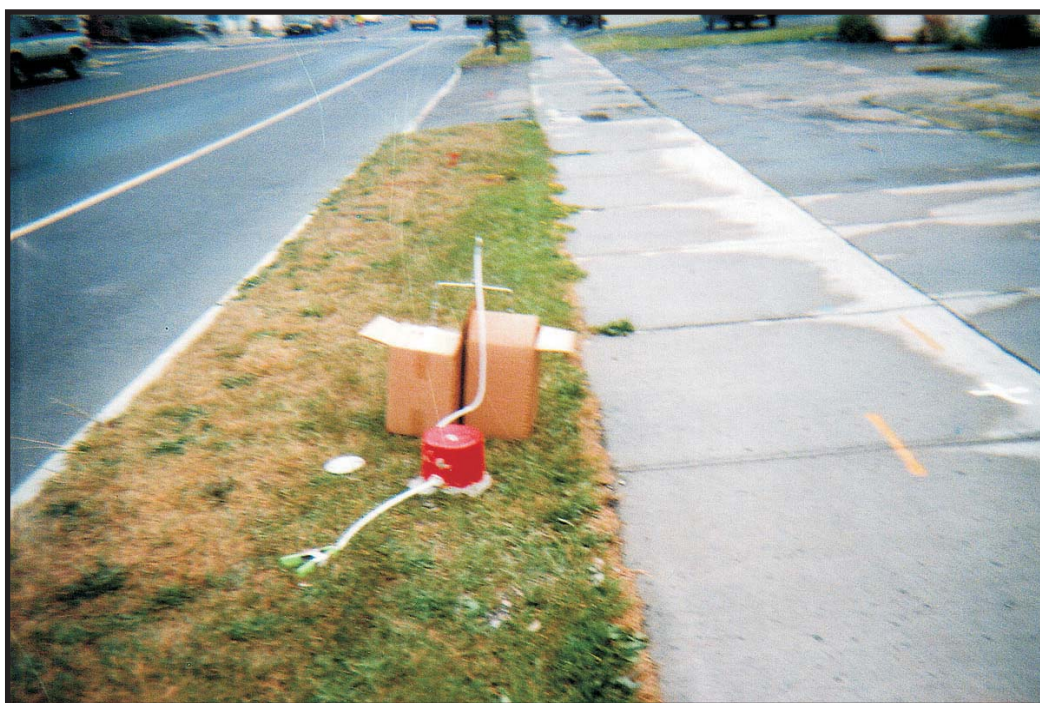
Photo 23: Photograph looking south at tracer gas and summa canister set-up at SG-6 location.
