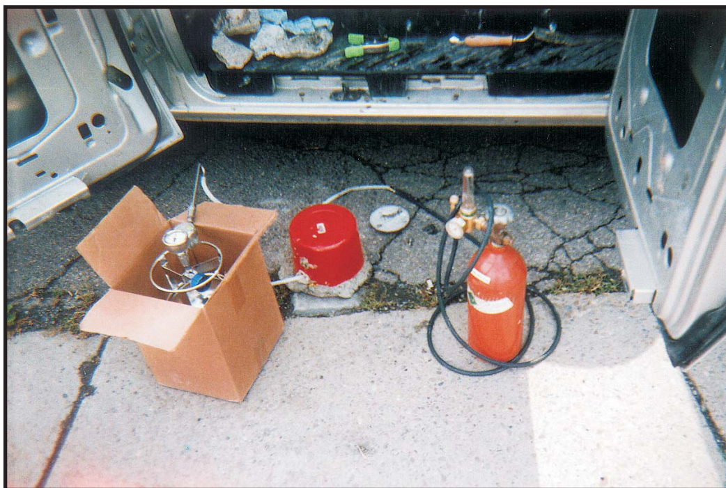
Photo 21: Photograph looking west at tracer gas and summa canister set-up at SG-4 location.
