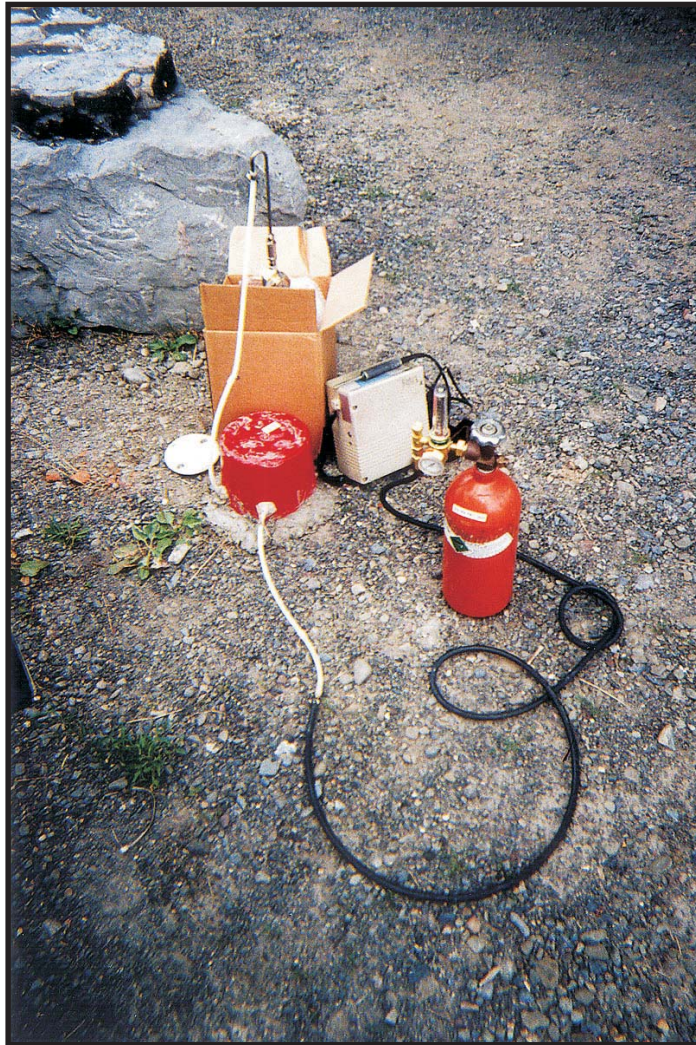
Photo 28: Photograph looking north at tracer gas and summa canister set-up at SG-11 location.
