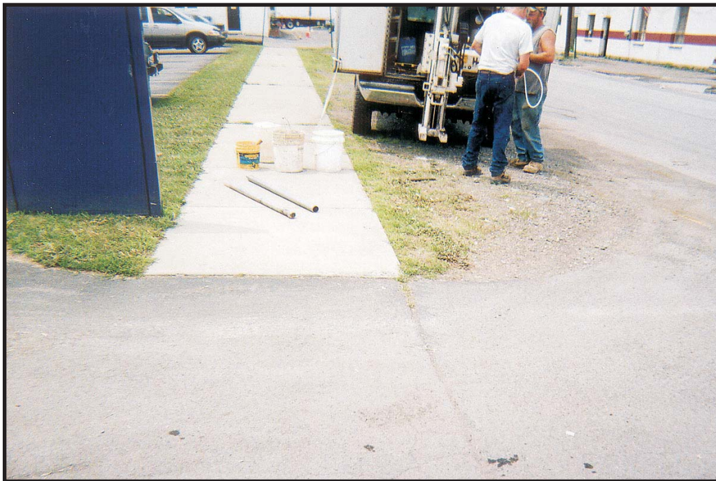
Photo 2: Geoprobe operators attaching polyethylene tubing to the soil gas implant.
