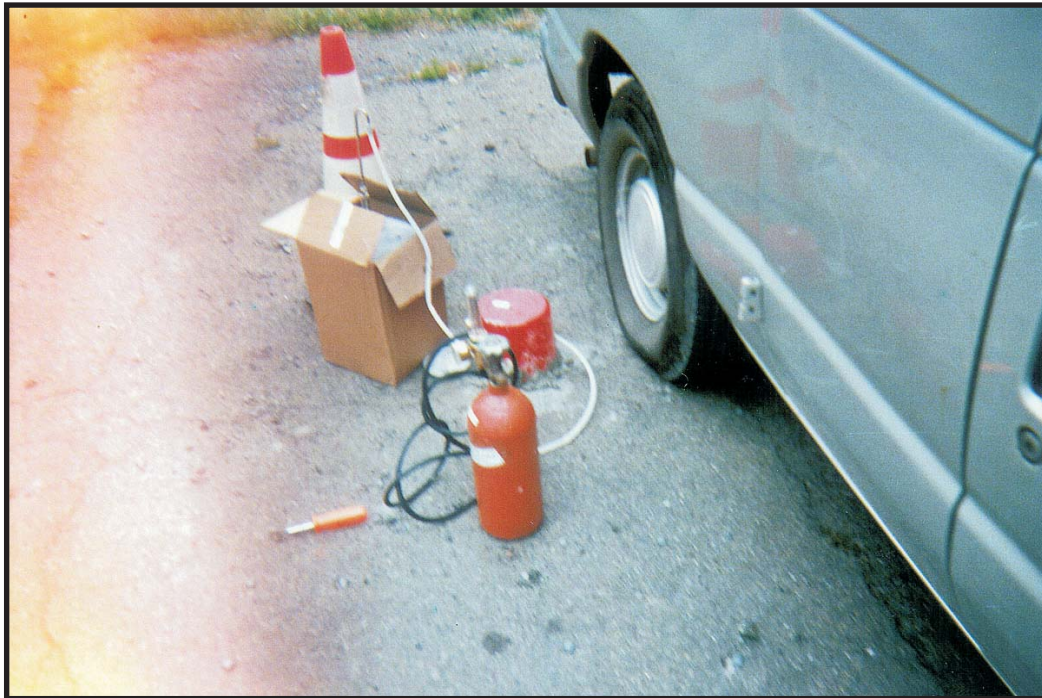
Photo 24: Photograph looking southwest at tracer gas and summa canister set-up at SG-7 location.
