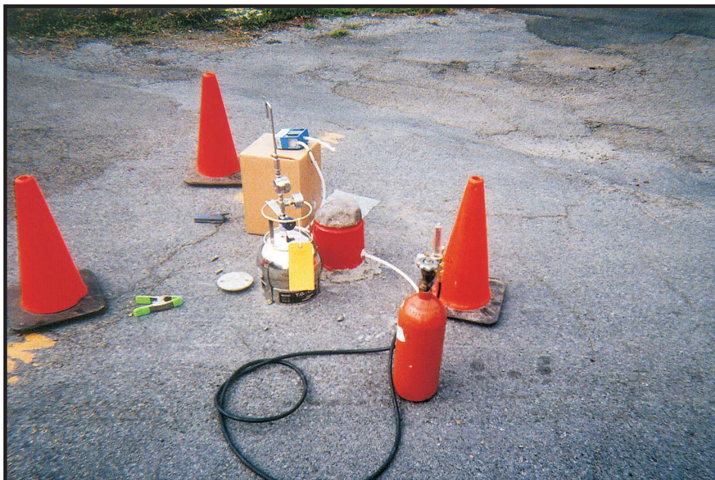
Photo 20: Photograph looking west at tracer gas and summa canister set-up at SG-3 location.
