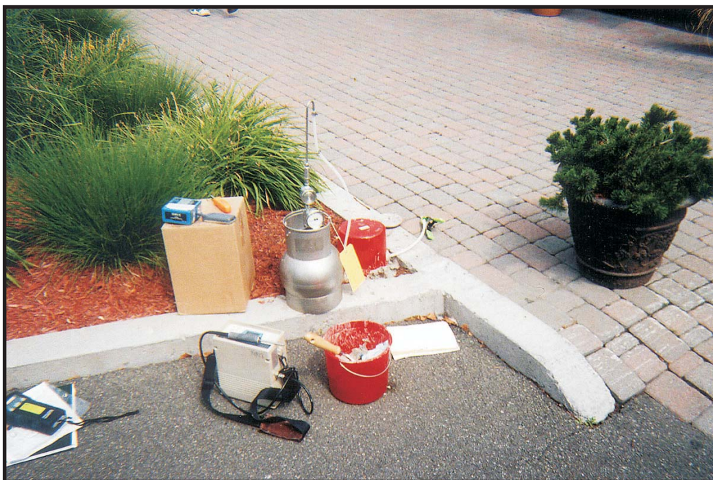
Photo 19: Photograph looking northwest at tracer gas and summa canister set-up at SG-2 location.
