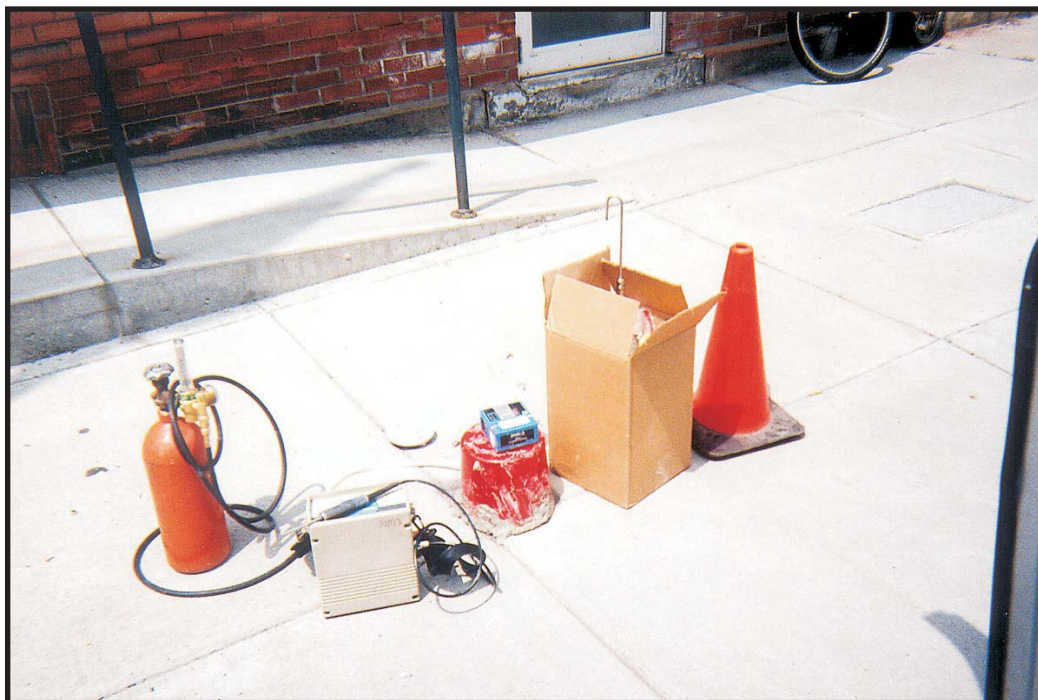
Photo 26: Photograph looking north at tracer gas and summa canister set-up at SG-9 location.
