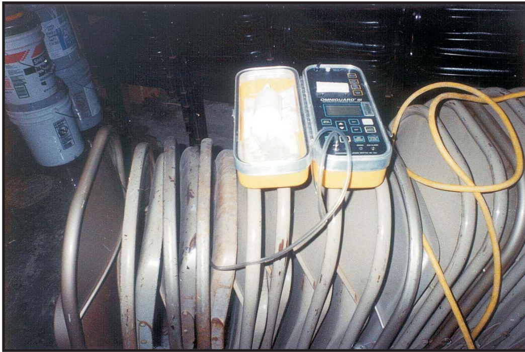
Picture of vacuum pressure gauge used to vacuum test.
