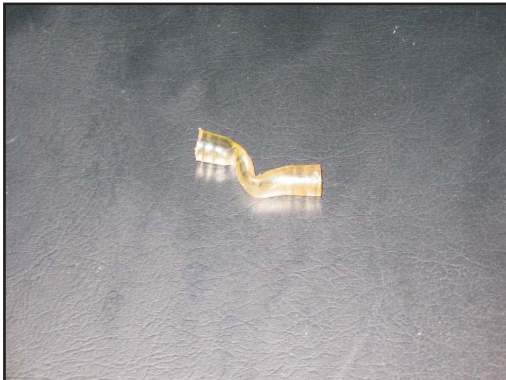
Photo 4: Crimped connection hose from suction point #1 magnehelic.
