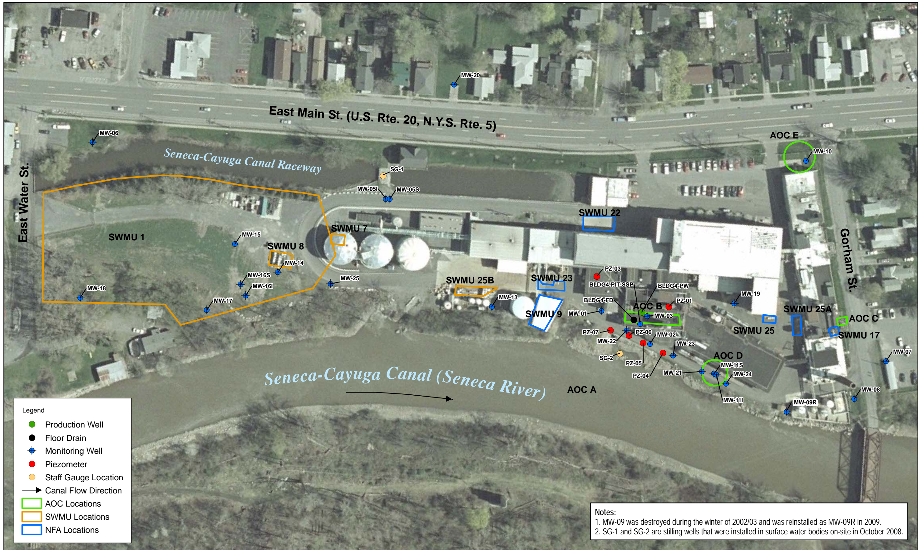
FIGURE 6 Groundwater and Surface Water Monitoring Locations Former Hampshire Chemical Corp Facility Waterloo, New York
