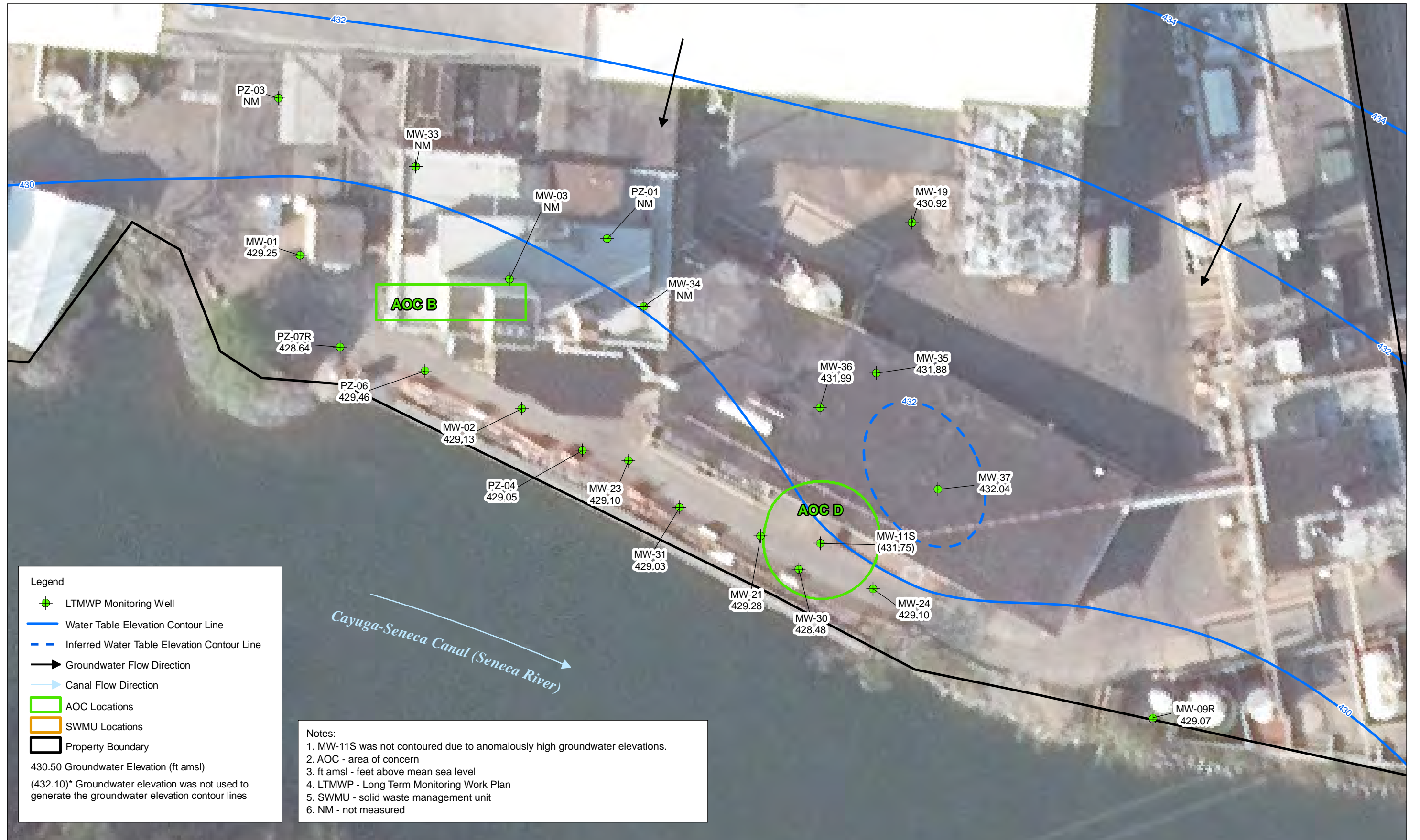
Figure 5-2 AOCs B and D Groundwater Elevation Contour Map, August 2017 2016 and 2017 Groundwater Monitoring Results and Year 2 Monitoring Natural Attenuation Performance Evaluation Report Former Hampshire Chemical Corp. Facility Waterloo, New York
