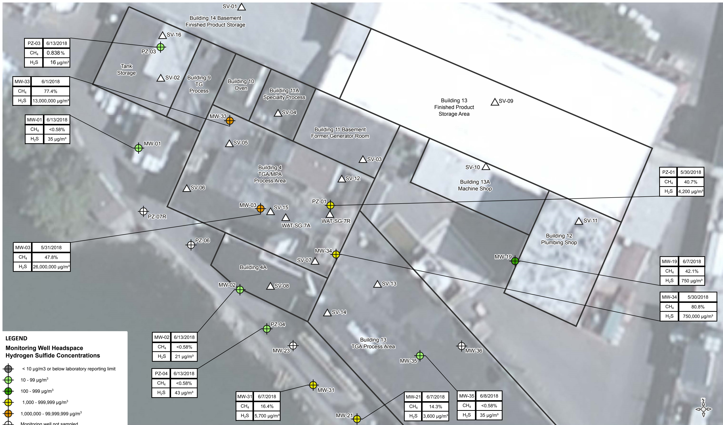
FIGURE 11-9 Monitoring Well Headspace Hydrogen Sulfide Results, May & June 2018 2018 Supplemental Building 4 Vapor Investigation Former Hampshire Chemical Waterloo, New York
