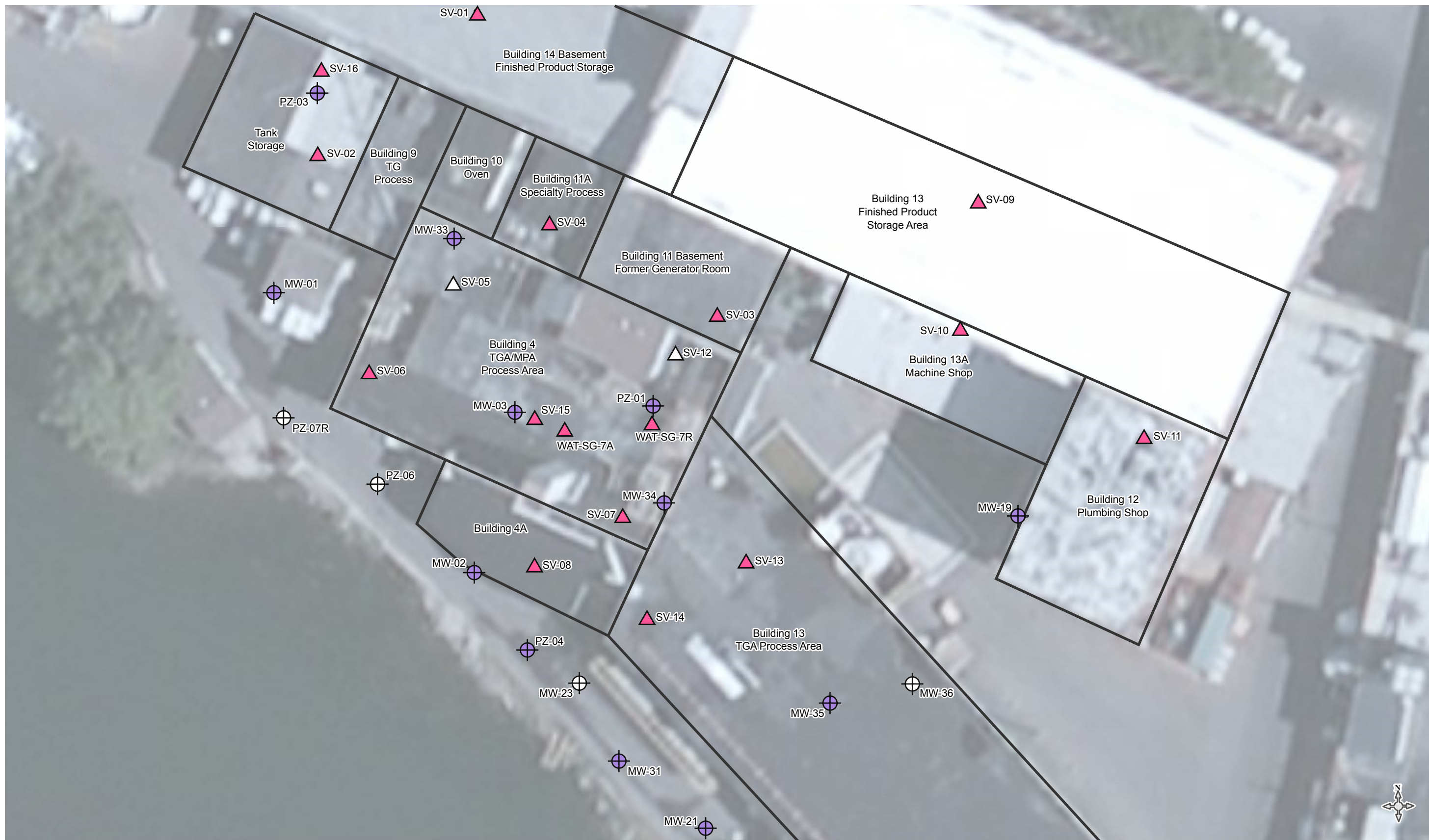
Figure 2-2 2018 Subslab and Headspace Vapor Sampling Locations 2018 Supplemental Building 4 Vapor Investigation Former Hampshire Chemical Waterloo, New York
