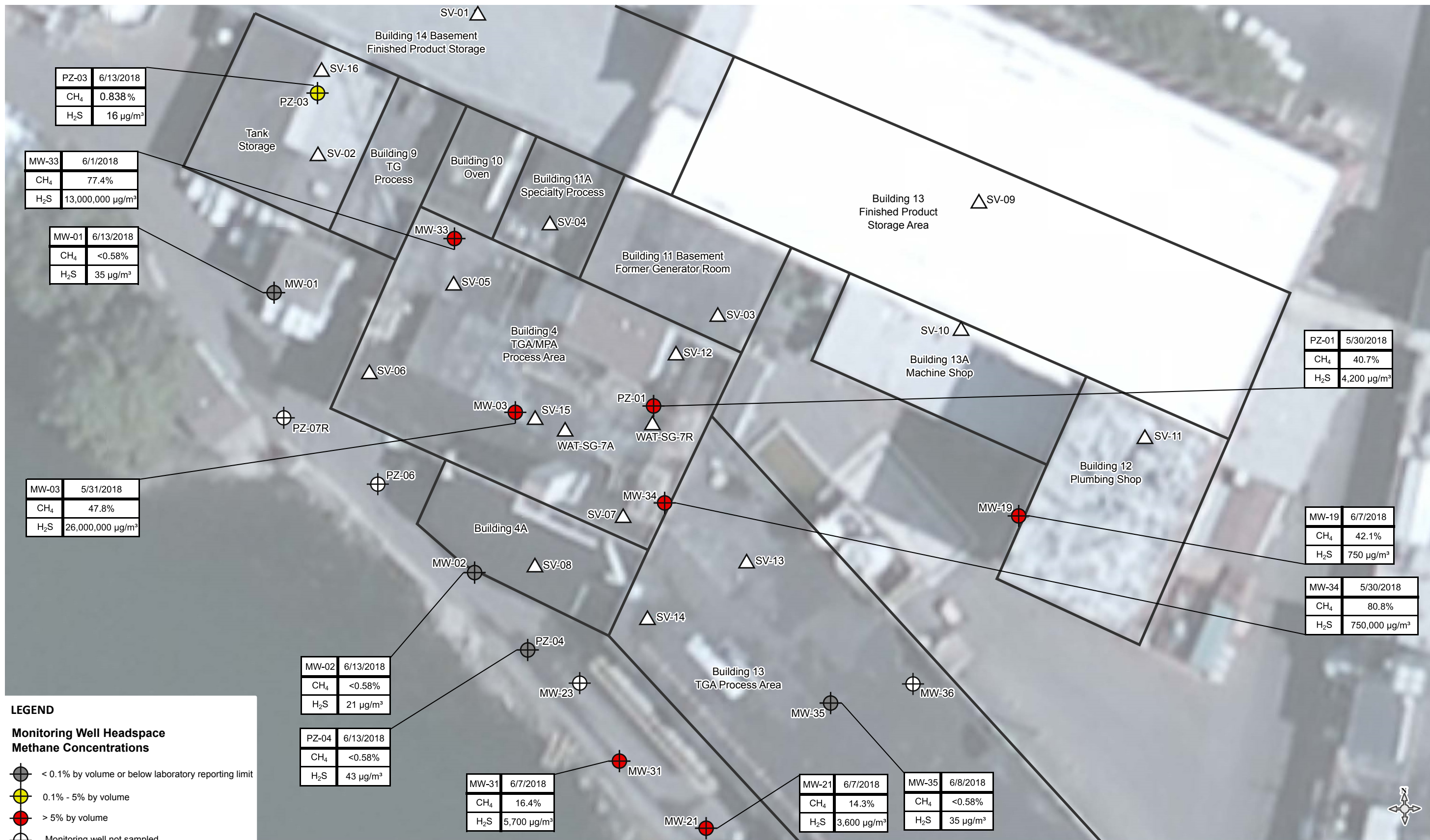
FIGURE 11-5 Monitoring Well Headspace Methane Results, May & June 2018 2018 Supplemental Building 4 Vapor Investigation Former Hampshire Chemical Waterloo, New York
