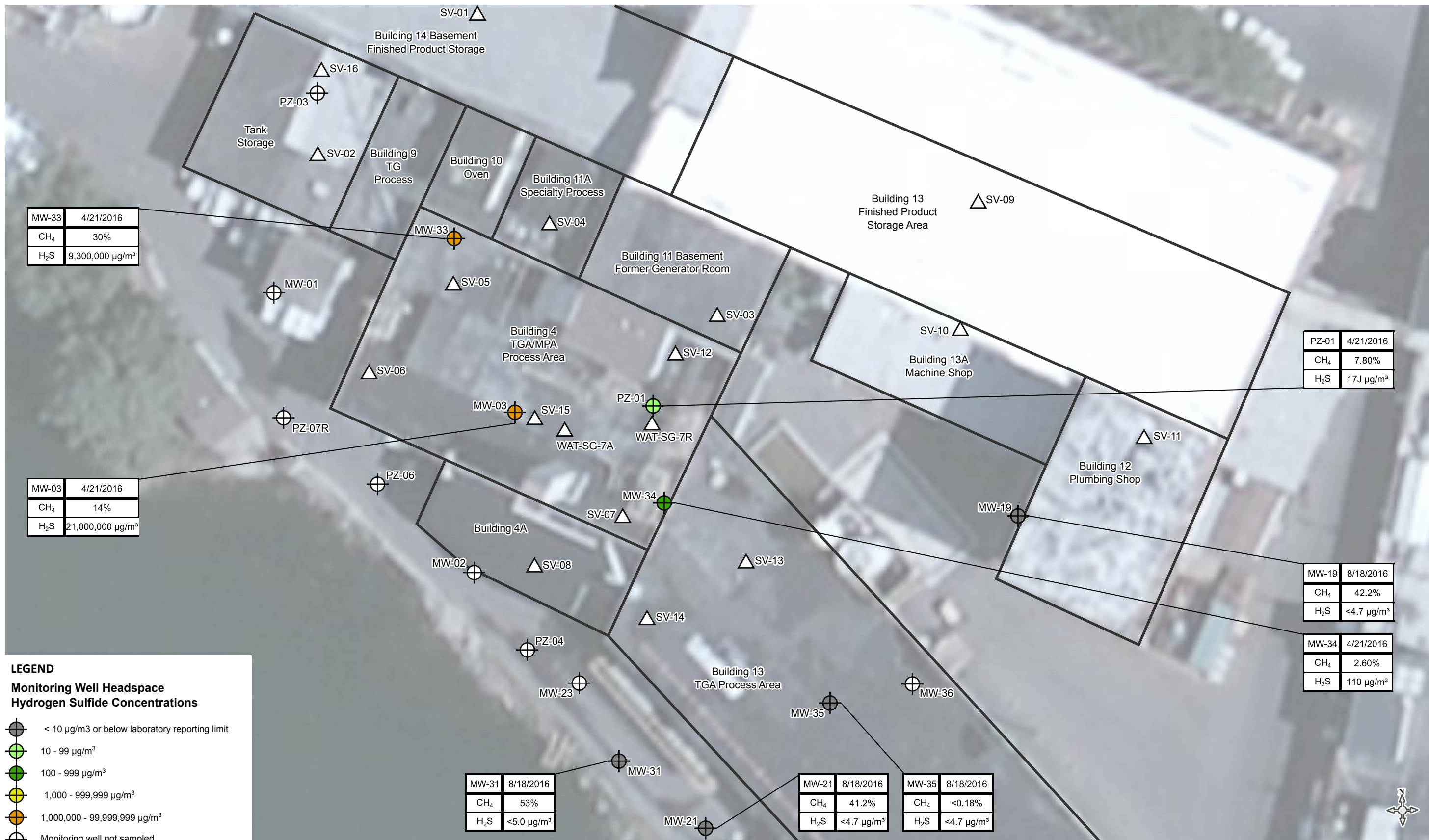
FIGURE 11-6 Monitoring Well Headspace Hydrogen Sulfide Results, April & August 2016 2018 Supplemental Building 4 Vapor Investigation Former Hampshire Chemical Waterloo, New York
