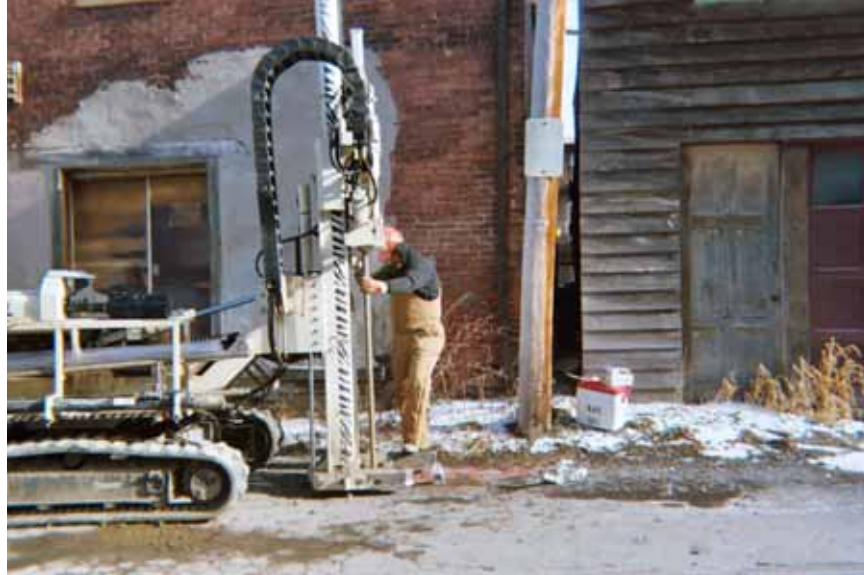
Date: 1/16/06 Subject: Direct-Push activities at the Band Box Cleaners Photographer: Jim Mays Site boring BB-BH-04
