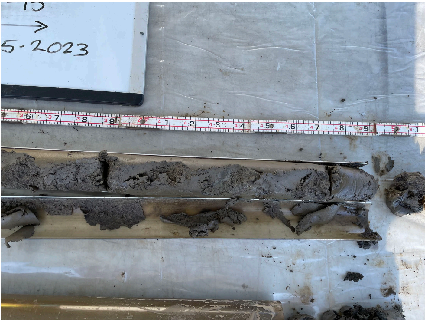
SB23 13-15 ft. bgs silty sand with light black staining
