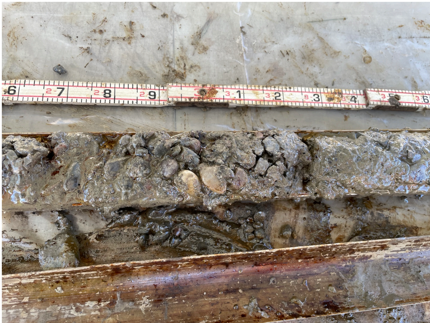
SB-23 \approx 42 ft. bgs Silty sand with gravel and heavy coating. Strong MGP odor.
