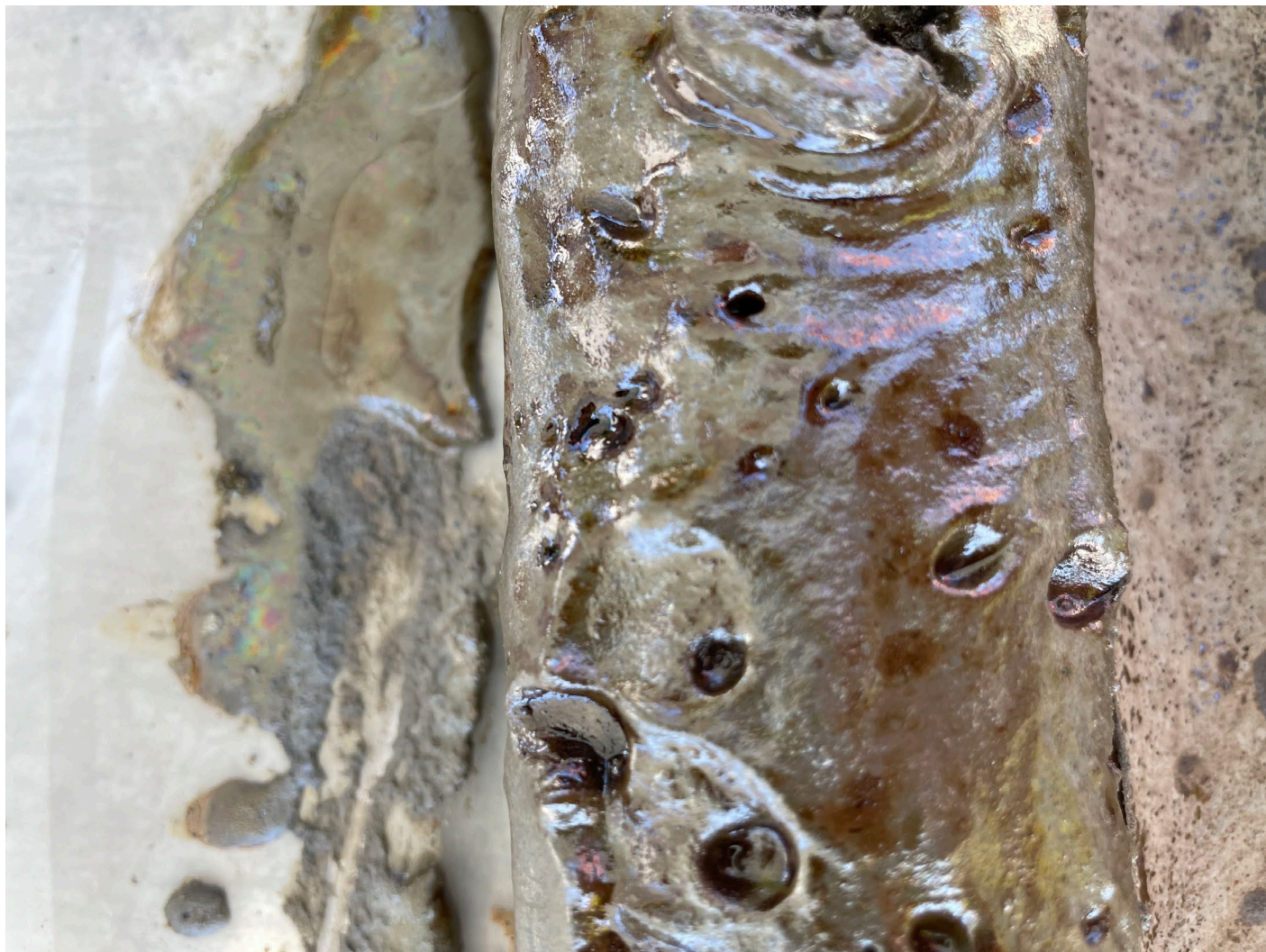
SB-14 ≈22 ft. bgs Wet silty-sand with blebs/NAPL 682 ppm VOCs
