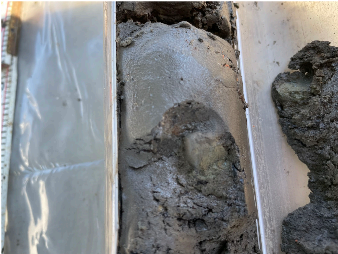
SB-23, ~10 ft. bgs, silty sand with trace cobbles and slight sheen
