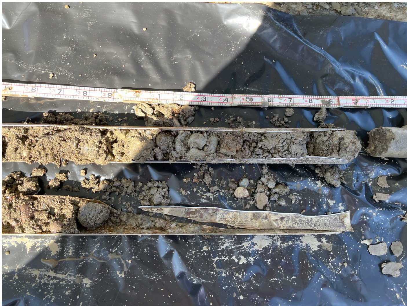
SB-14 \approx 14 ft. bgs moist sand with gravel and cobbles. Lightly coated and moderate MGP odor. 659.8 ppm VOCs.
