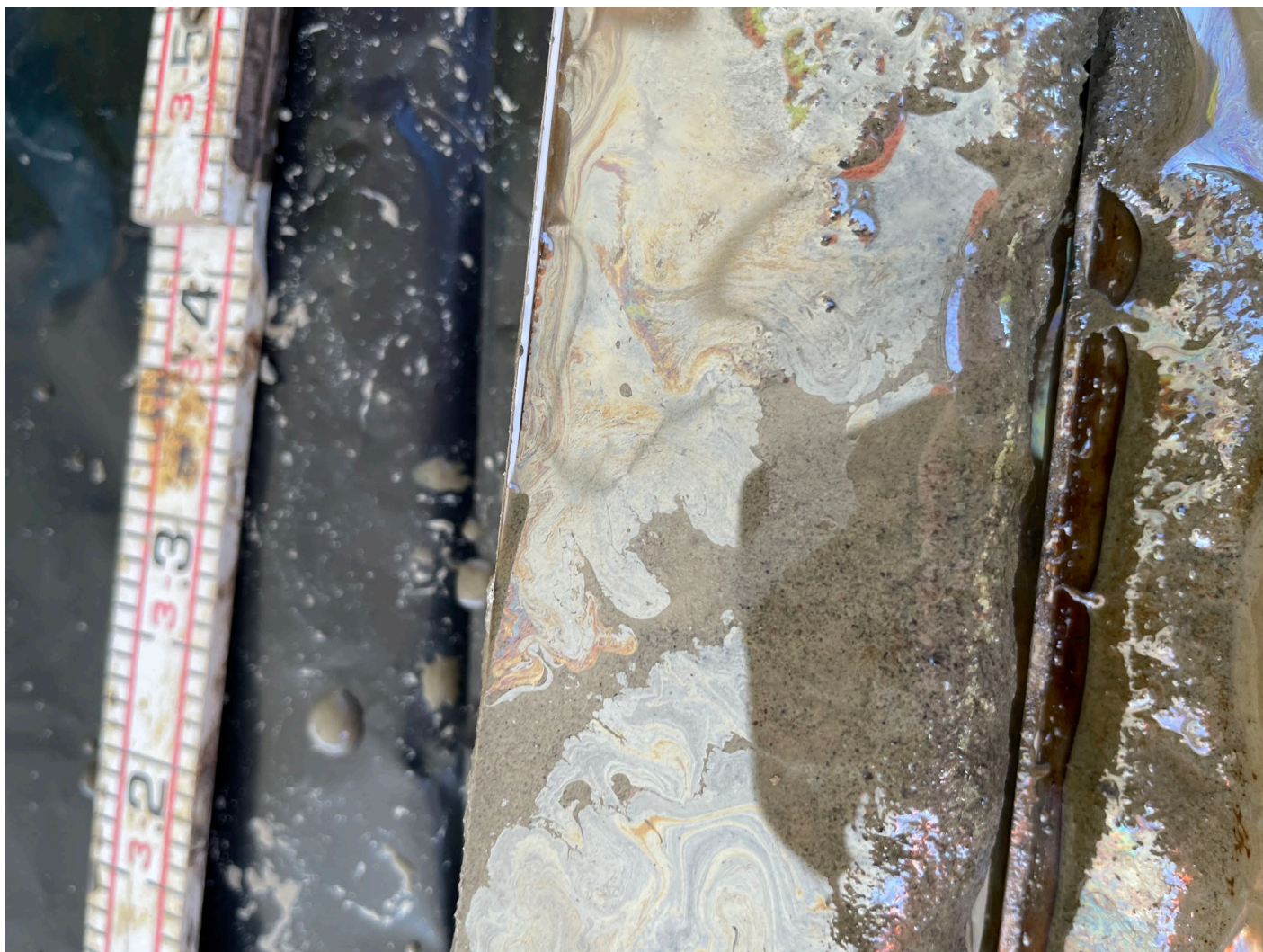
SB-14, \approx 47 ft. bgs wet, poorly graded, very fine sand with sheen
