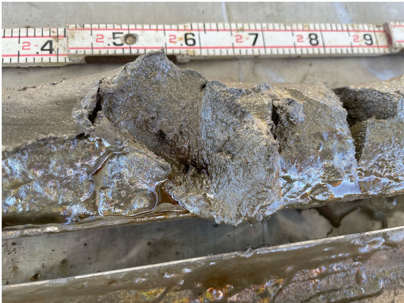
SB-23 ≈22 ft. bgs. gray, wet sand with sheen and moderate coating
