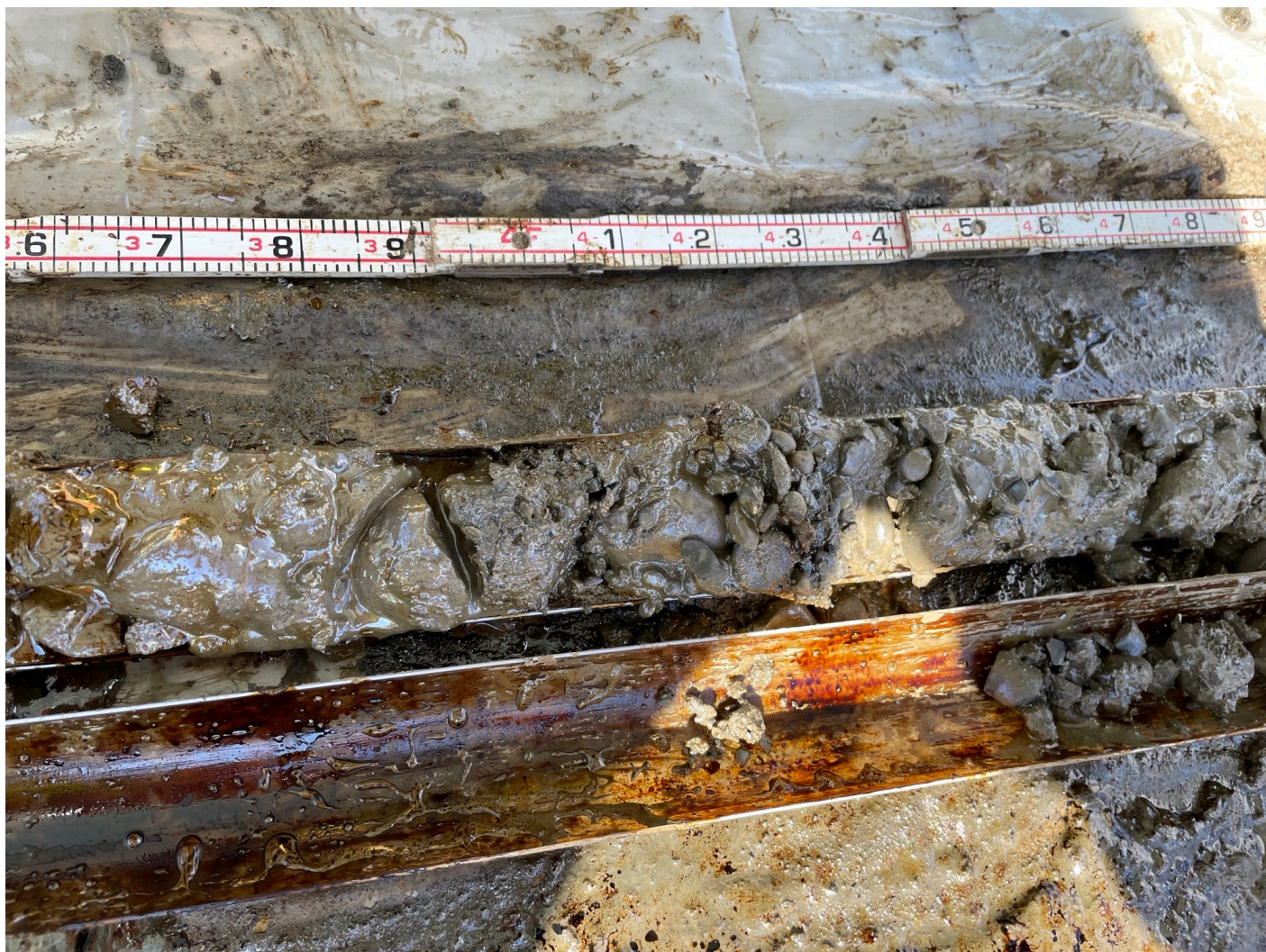
SB-23 ≈39 ft. bgs wet gray silt with gravel and moderate coating
