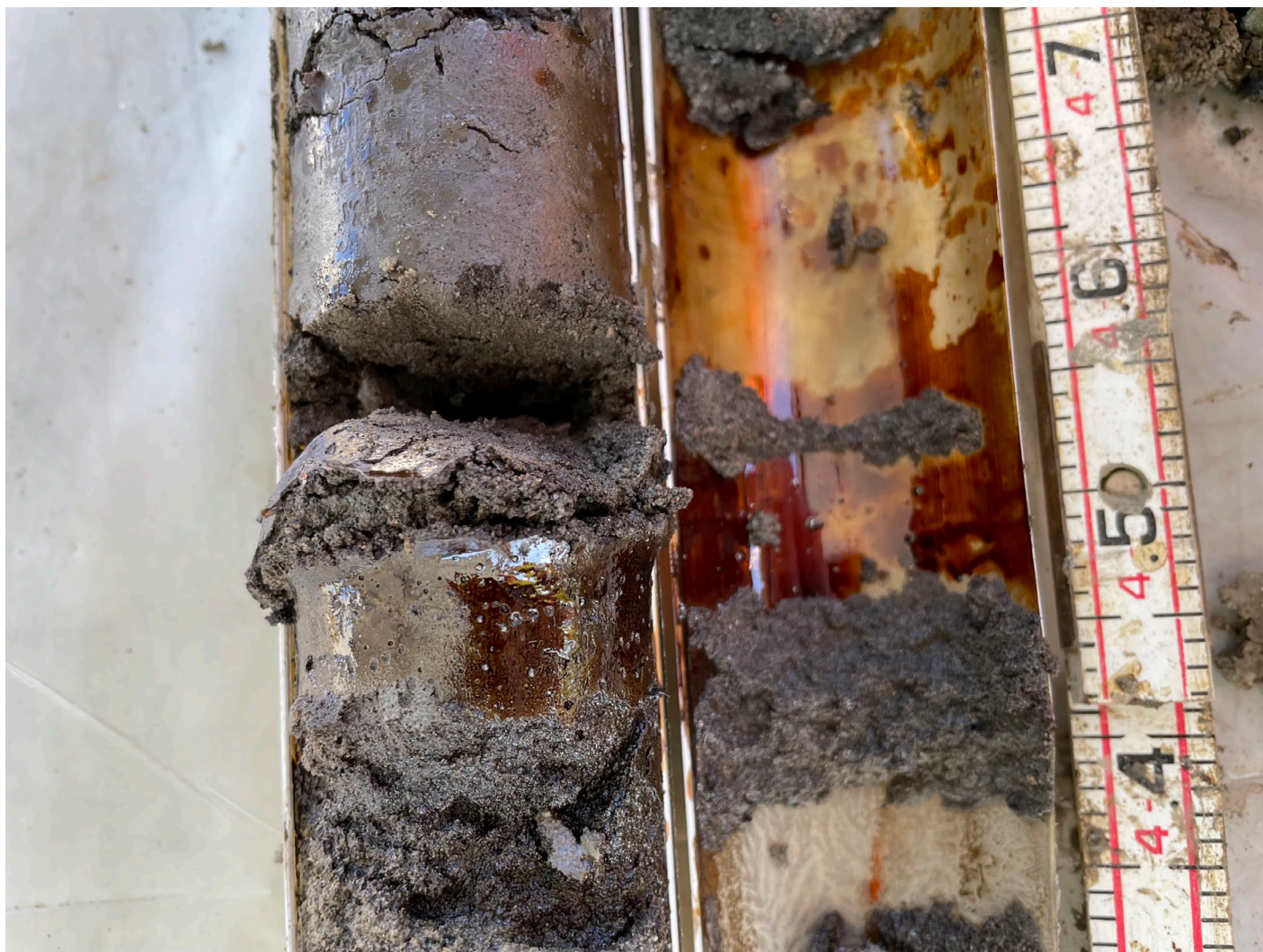
SB-14 \approx 19.5 ft bgs. Wet, clayey sand with narrow band of saturation/NAPL. 68 ppm VOCs.
