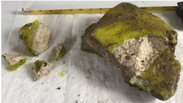
Picture 23: Uranium glass fused to refractory brick.
