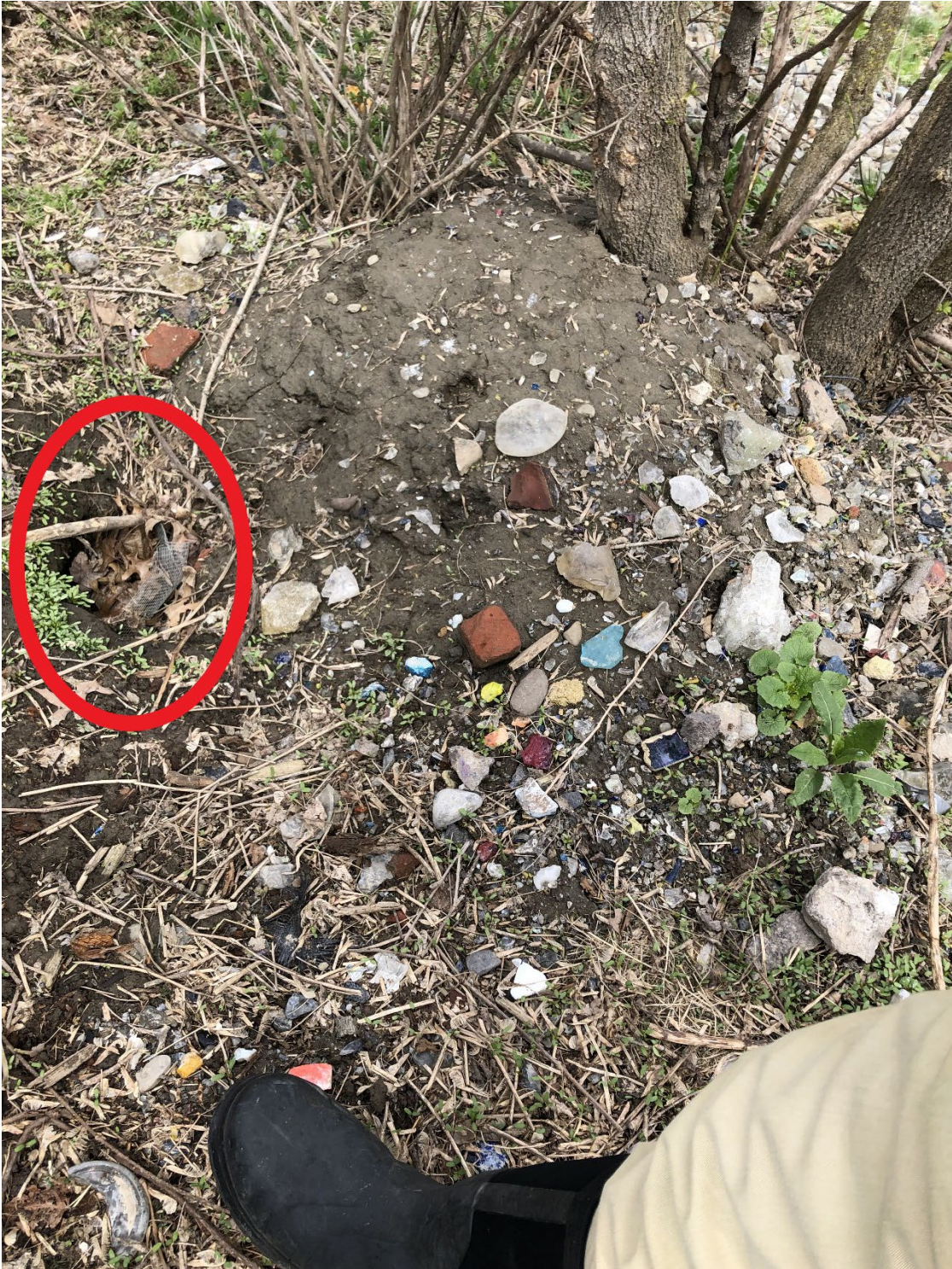
Picture 25: Comingled red brick, refractory chunks, and cullet. ABG ejected from animal burrow (circled red).
