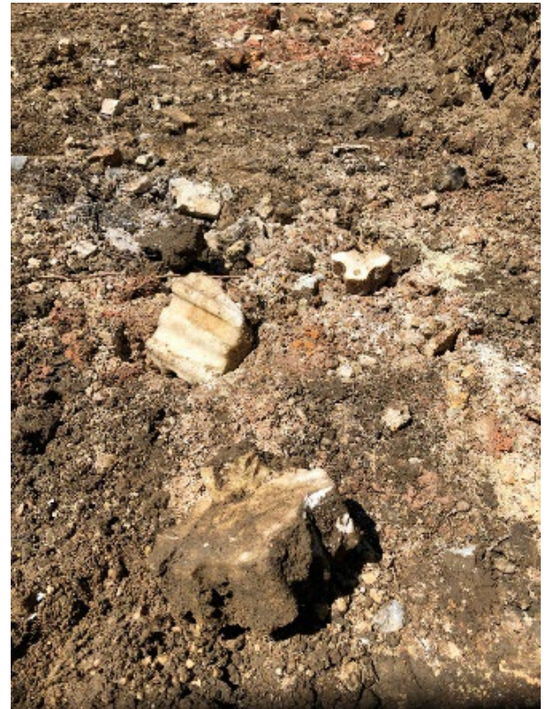
Picture 1: Primarily ash and brick in a 2-ft excavation.
