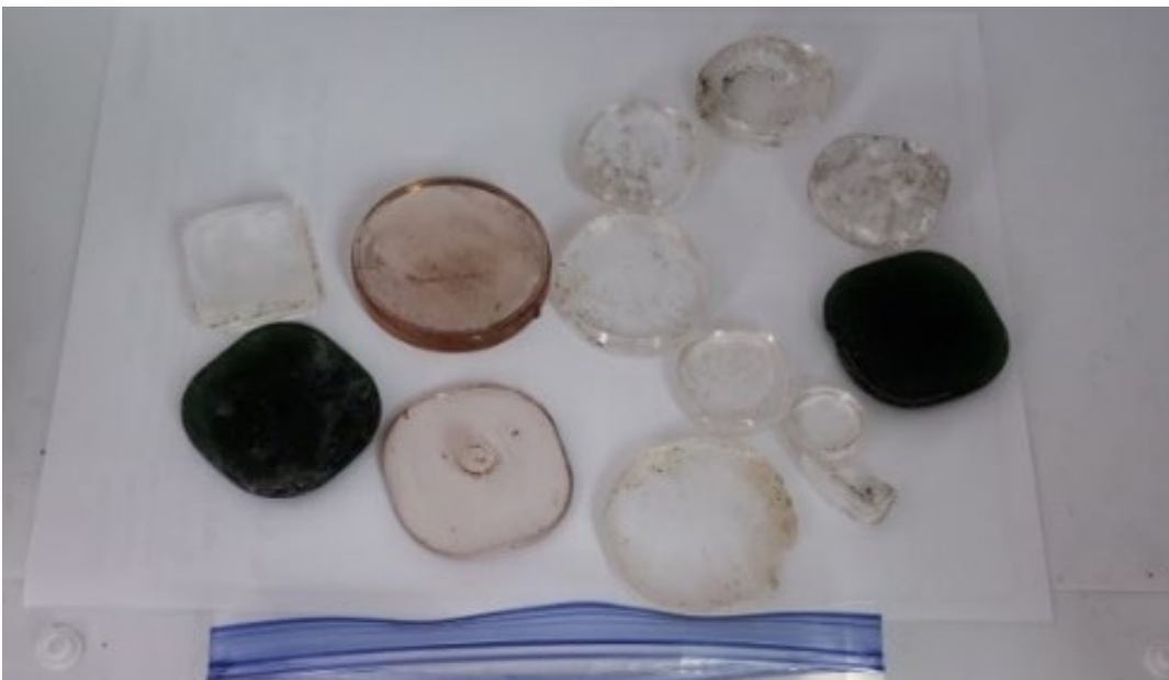
Picture 18: Green, light brown, and clear optical and ophthalmic lens blanks of various shapes.
