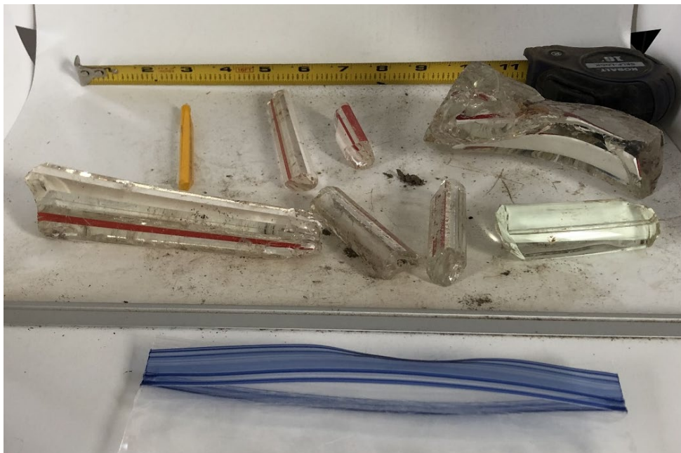
Picture 9: Most thermometer tubing fragments have strips of white and red glass encased in clear glass. One piece has an orange strip (top left). One piece has only a white strip (bottom right).
