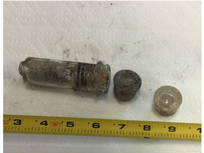
Picture 19: Insulator (left) and two glass fuses. “PYREX” is embossed on each piece.
