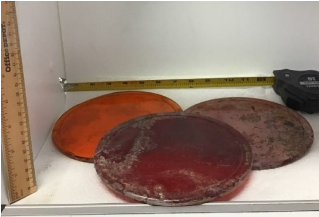
Picture 17: One orange and two red disk lenses. Each lens is embossed along the rim with "CORNING T. M. REG. U. S. PAT. OFF. MADE IN USA."
