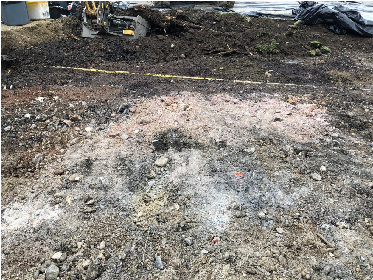
Picture 26: Comingled black ash and slag (top, along yellow gas line), cullet, refractory pieces, gray ash, and light orange ash.
