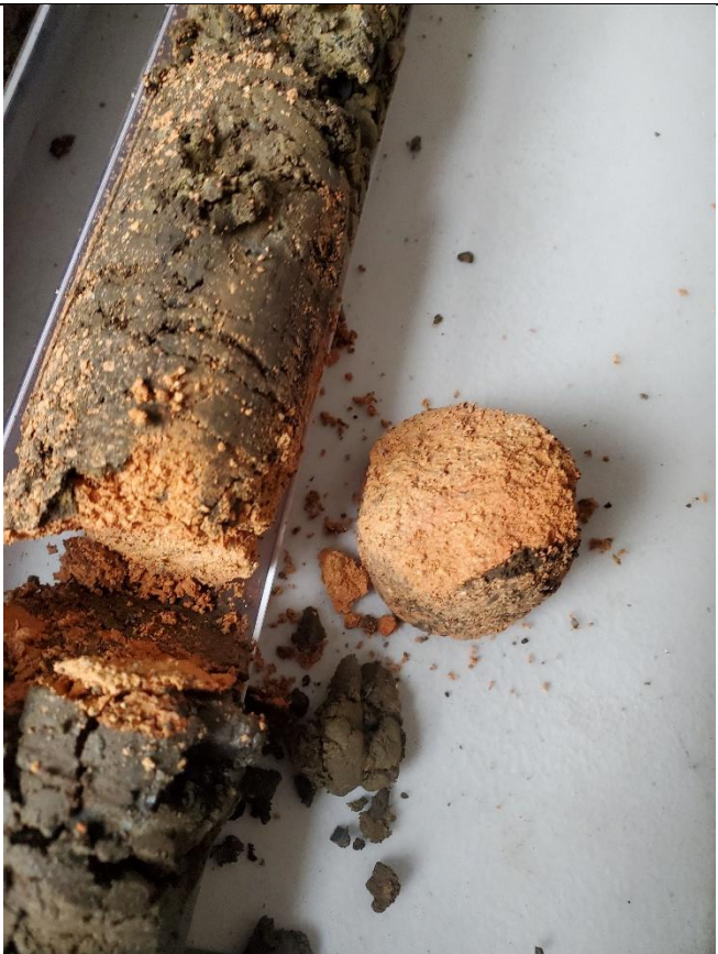
Picture 16 SS-10 close up of tan probable furnace brick
