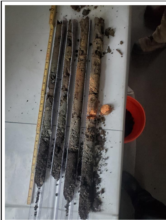
Picture 15 SS-10 cores with visible probable furnace brick from 1-1.3 FT BGS in one core.
