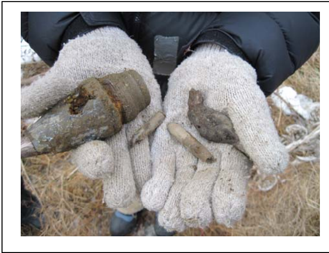
TP06 - projectile fuze, 50 caliber small arms casings
