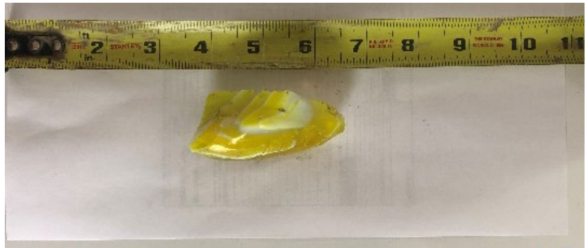
Picture 5: Cullet with layers of yellow and white.
