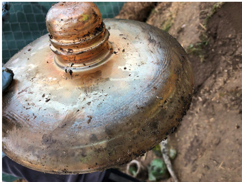
Picture 21: Opalescent insulator with approximately 1-ft diameter.
