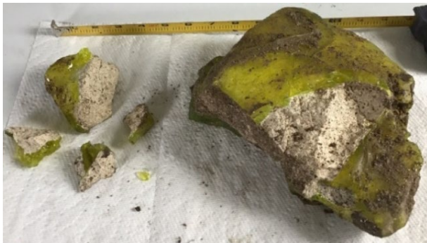
Picture 23: Uranium glass fused to refractory brick.
