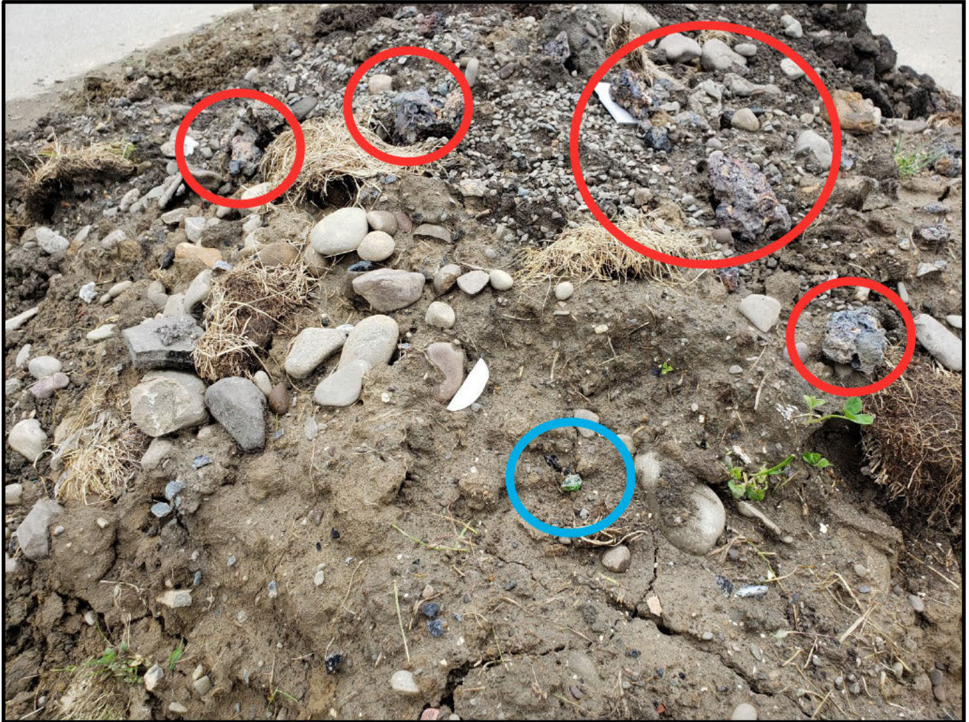
Photograph 3: A close-up of a spoils pile generated at Townsend Avenue in May 2022. A piece of green cullet (circled in blue) and chunks of slag (circled in red) are present on the surface of the spoils pile.
