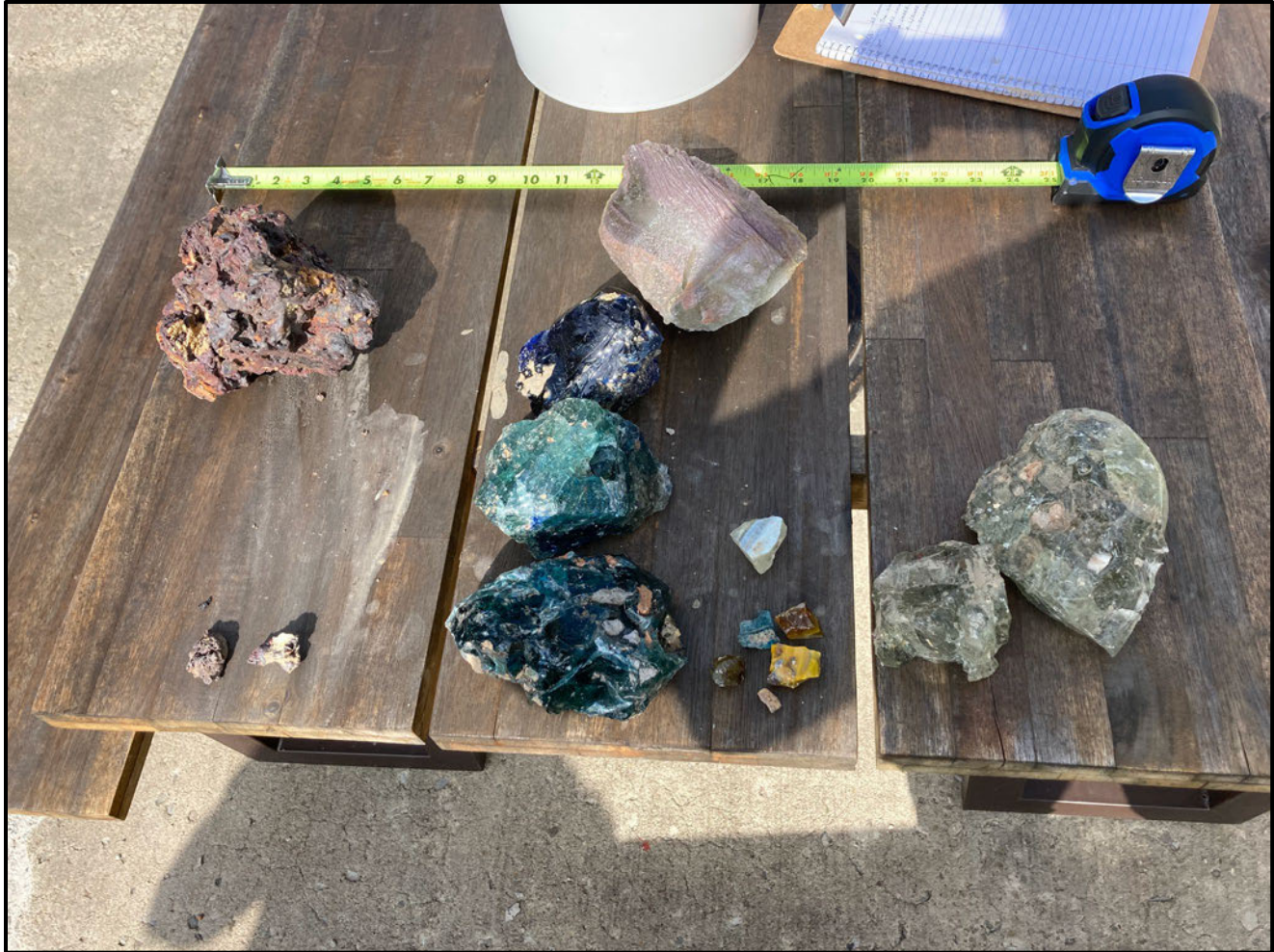
Photograph 1: Glass cullet (center and right) and slag (left) collected by the property owner from excavated portions of Townsend Avenue, Corning, New York. Of the three larger blue cullet chunks, the top and bottom appear to be glass fused to refractory material. Buff-colored material appears to underly the glass as shown by obtrusions of buff-colored material on the sides of the cullet pieces.
