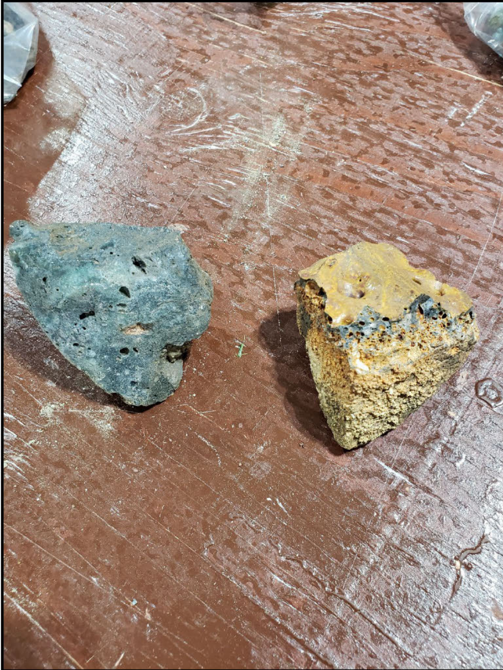
Photograph 5: Two chunks of glass fused to refractory collected by the property owner from the spoils pile in May 2022.
