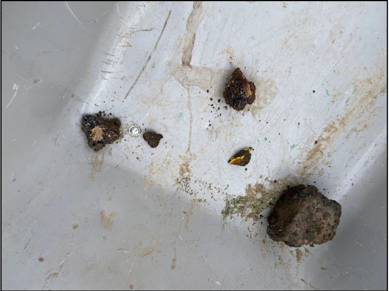
Photograph 6: Slag (left), yellow cullet (center right), and brick (bottom right) excavated from a hand-cleared location at Townsend Avenue on October 19, 2022.
