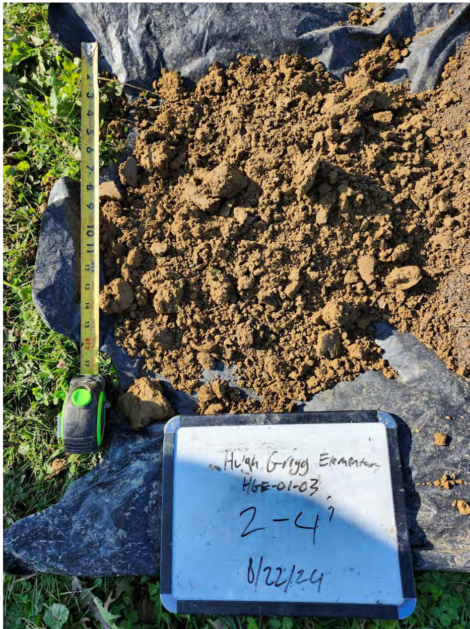
Image of soils from boring location HGE-01-03 (Hugh Gregg Elementary School). The pile of soil in the image contains soil collected from the 2 to 4-foot interval. No ABG was observed in this interval.
