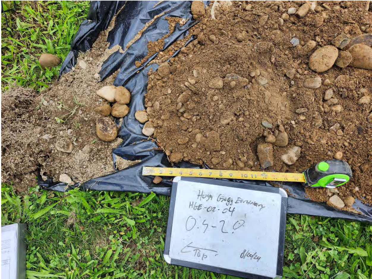
Image of soils from boring location HGE-02-04 (Hugh Gregg Elementary). The pile of soil in the center left portion of the image contains soil collected from the 0.5 to 2-foot interval. Small brick fragments (non-ABG) were encountered below 1.25 feet in this interval.
