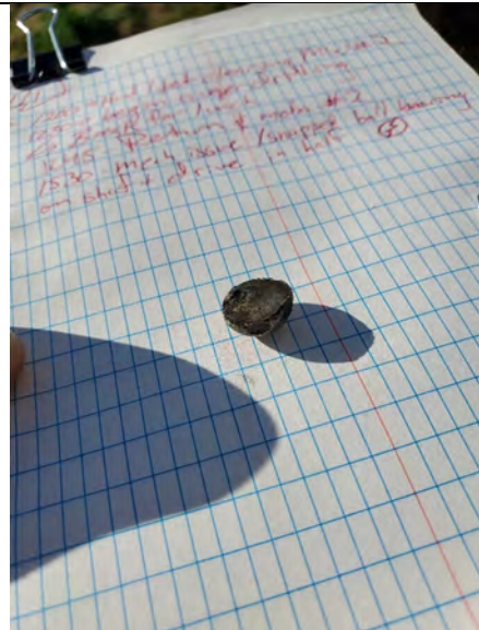
Photo 8: Sheered ball bearing from when mechanical issues arose at the B412-OW-D location.
