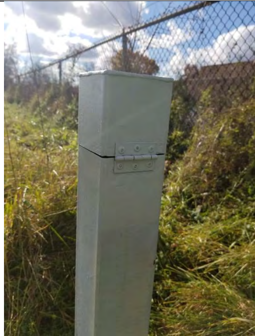
Photo 6: B103-OW-A's new cap and hinge; staged in the mount position.
