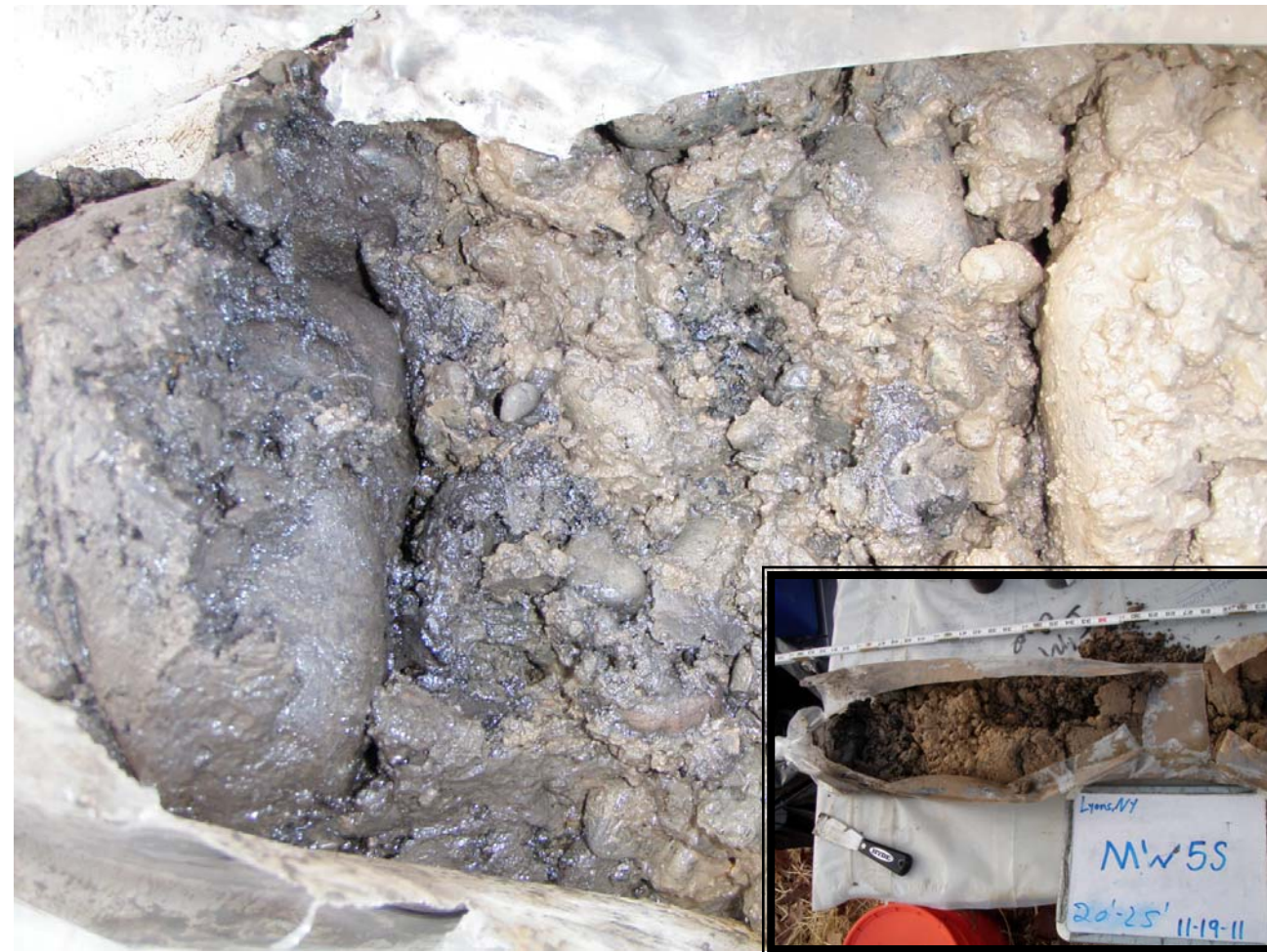
Photograph #1: Soil from soil boring MW5S from 24 to 25' bgs. Black hydrocarbon staining and soil coated with brownish-black tar-like material.
