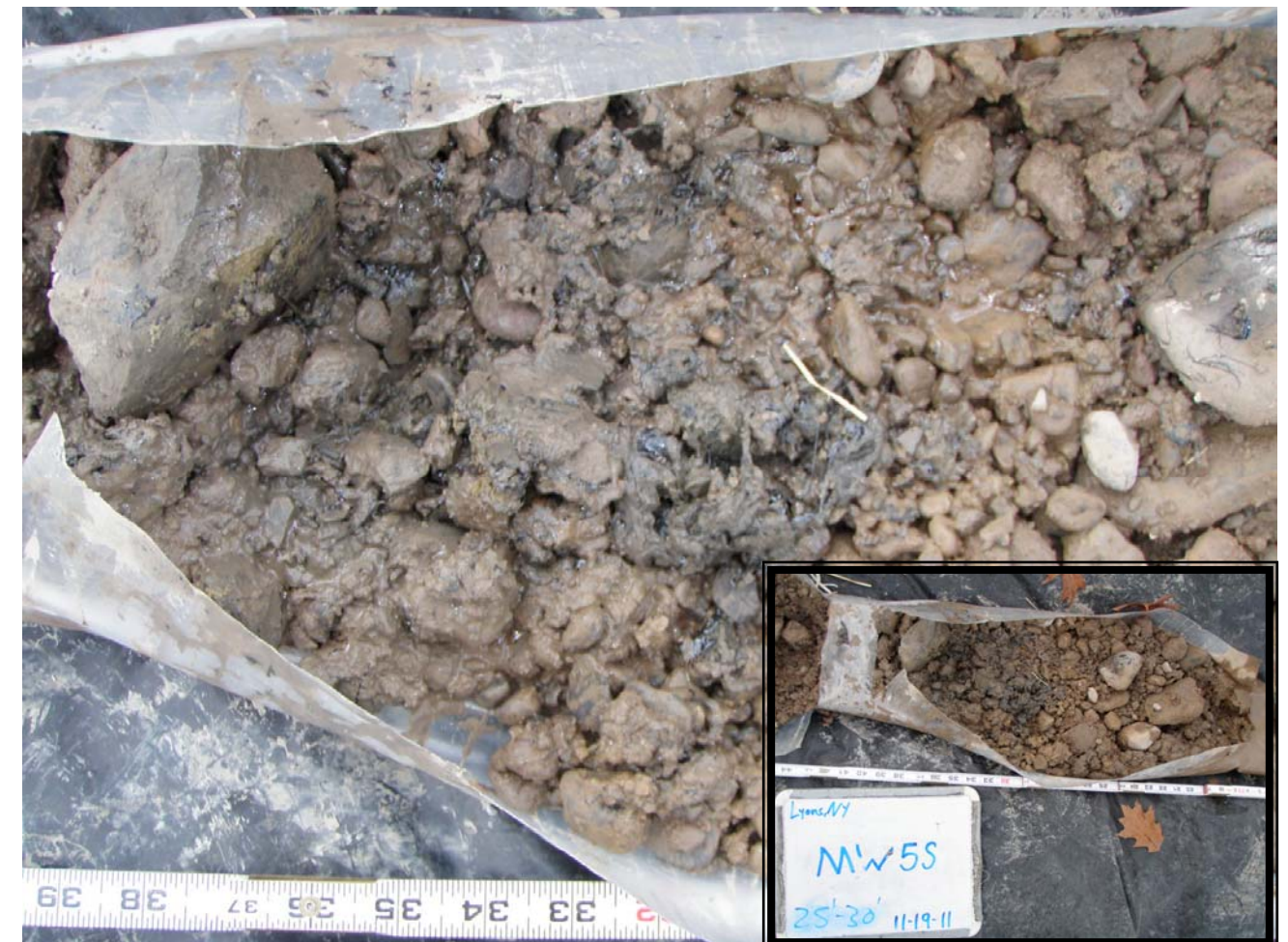
Photograph #2: Soil from soil boring MW5S from 26.8' bgs to 27.4' bgs. Soil coated with tar-like material.
