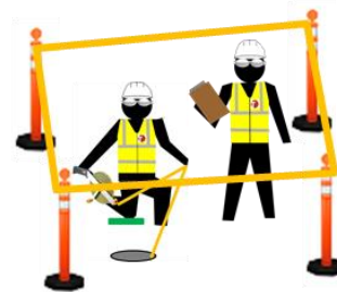
Scenario #2: Intermediate Term (1-8 Hours) Channelizing Cones with Caution Tape and Lookout
