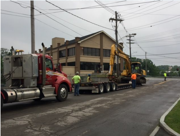
Demobilizing PC220 with Robovibe attachment following completion of structural sheetpile installation.
