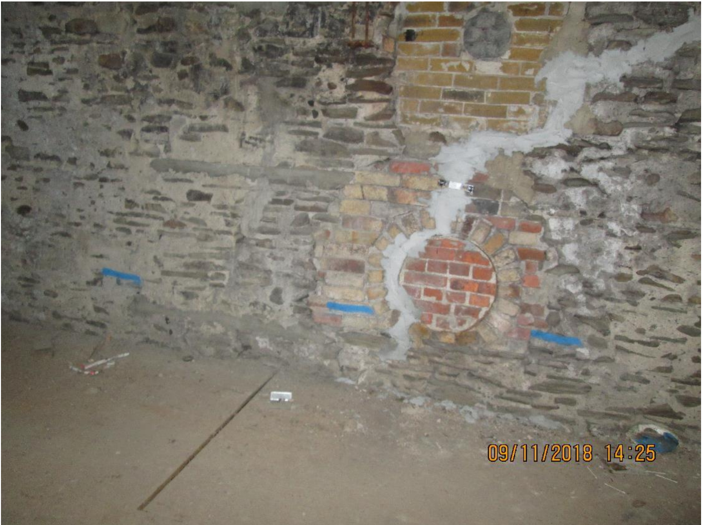
Photo 8: View of the level markings on the second floor of the MGP for AECOM's liquid level settlement system.
