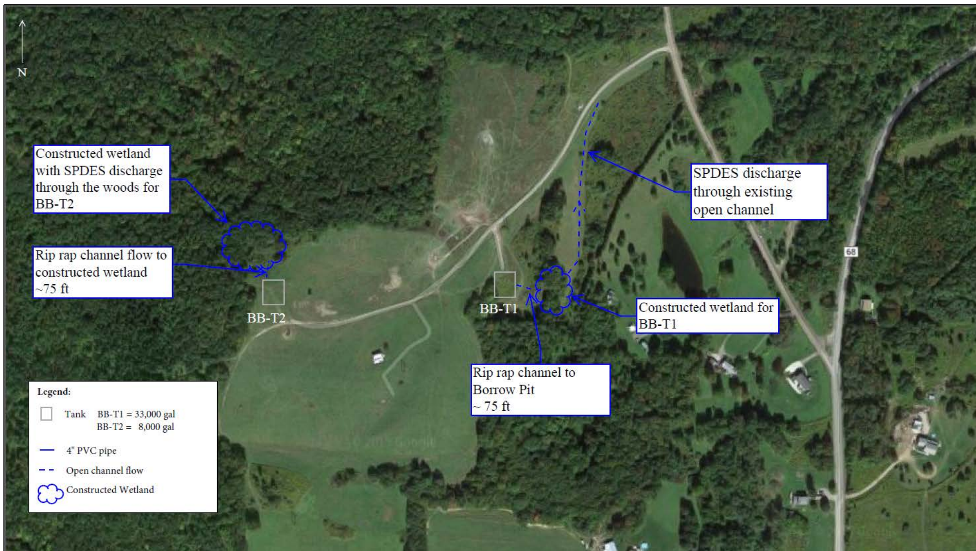
Figure 5 Alternative 4: Passive Treatment In Separate Constructed Wetlands
