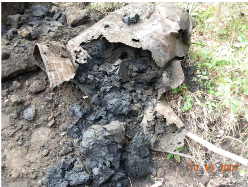
Contents of a 55-gallon drum encountered in Test Pit 10 (saturated, black fine sand material)
