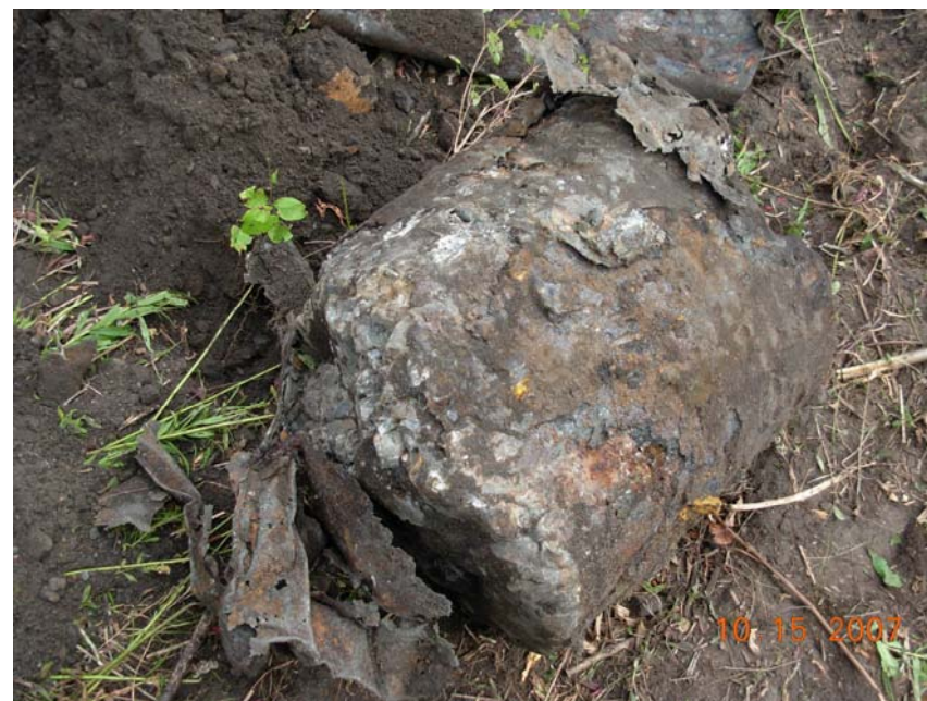
55-gallon drum excavated from Test Pit 2 (“whitish slag” material)
