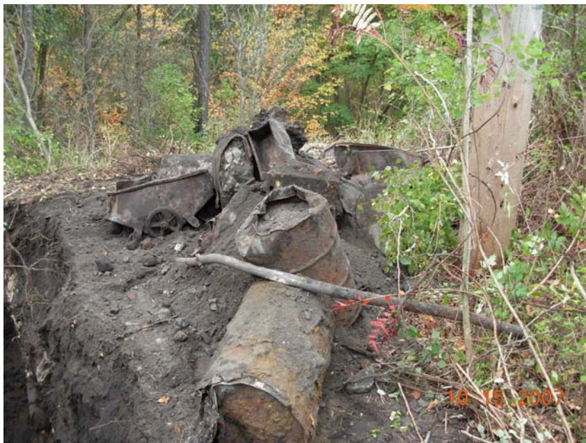
Debris from Test Pit 1 (i.e. drums, metal fragments, etc.)
