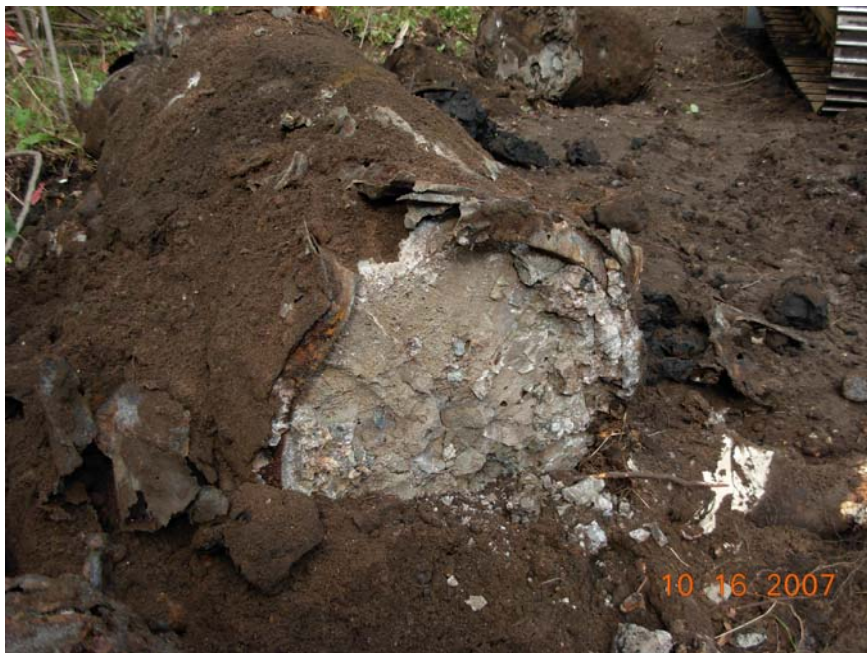
55-gallon drum encountered in Test Pit 10 (“whitish slag” material)
