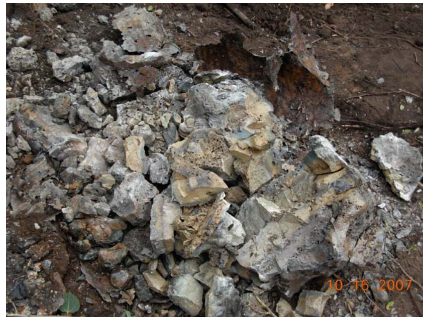
Contents of a 55-gallon drum encountered in Test Pit 10 (“tan resin” material).
