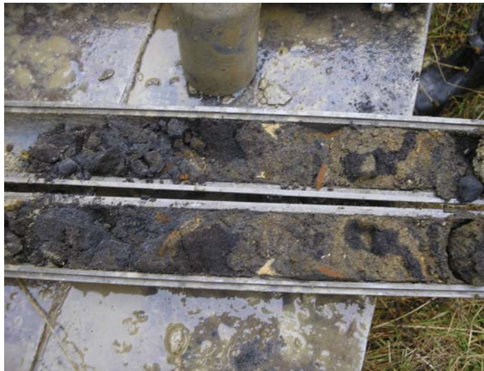
Foundry Sand Waste In Split Spoon Sample (Trench 3)
