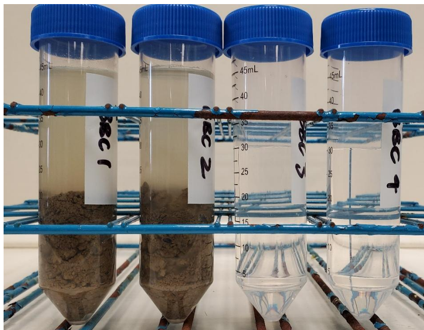
Picture 1: Base Buffering tubes before NaOH addition, groundwater control (no pH adjustment) on right
