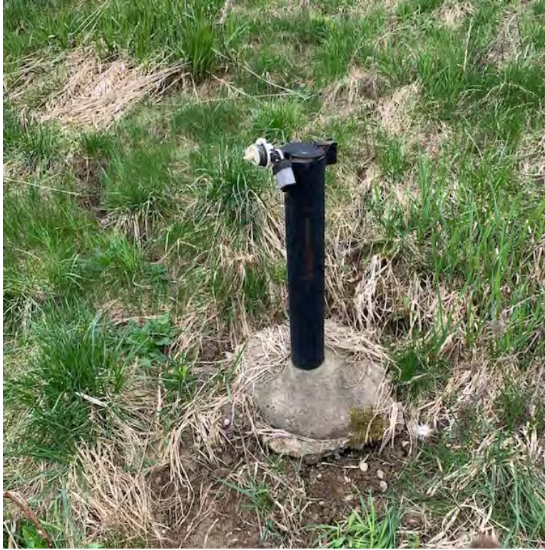
Photo 11 – MW-2S(R) with wrong size cap, MW-5S lid was locked by Great Lakes.
