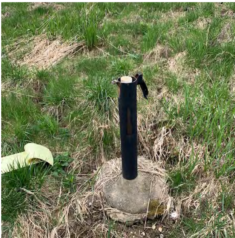
Photo 10 – MW-2S(R) found uncapped and unlocked.
