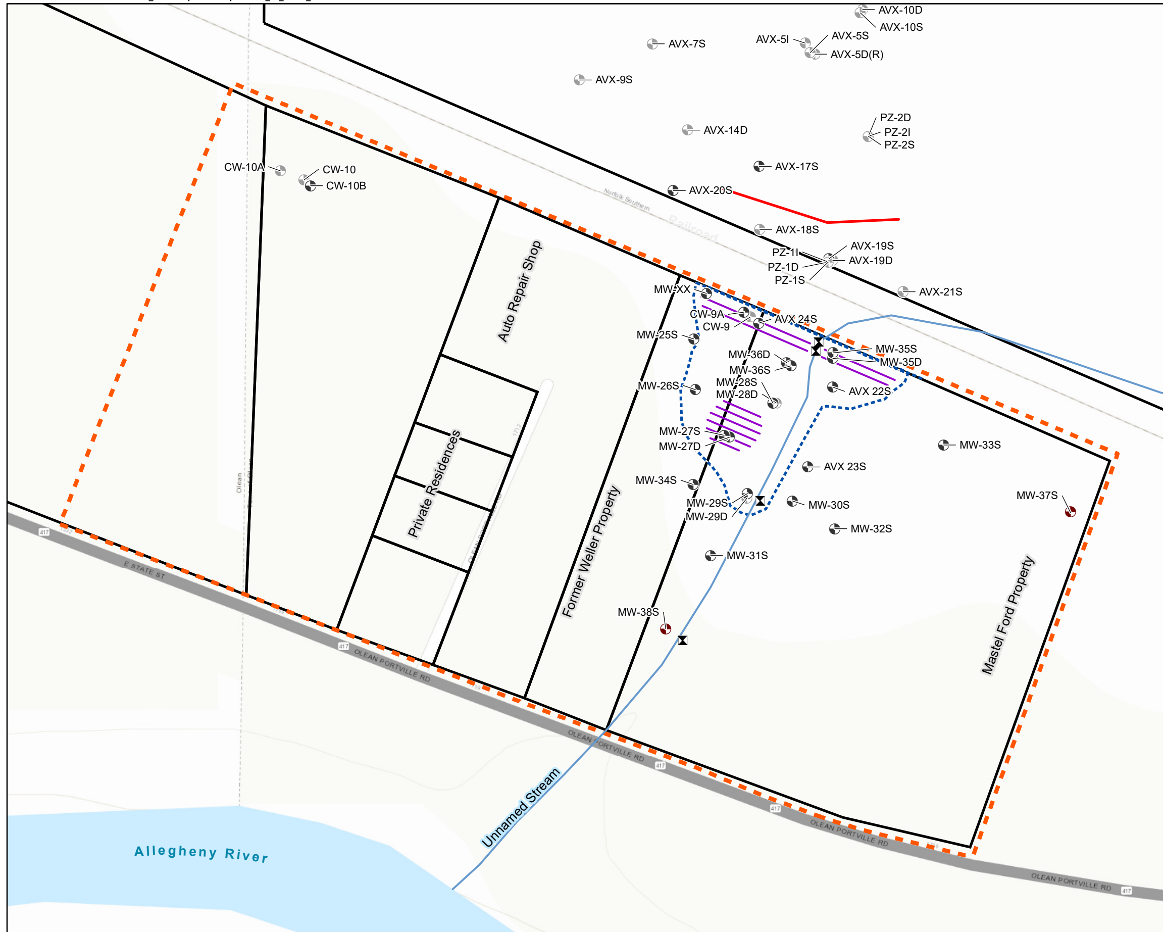
Figure 4-4 Olean Well Field OU4 Alternative 5: In-situ Chemical/Biological Treatment, Long-term Monitoring and ICs Cattaraugus County, NY
