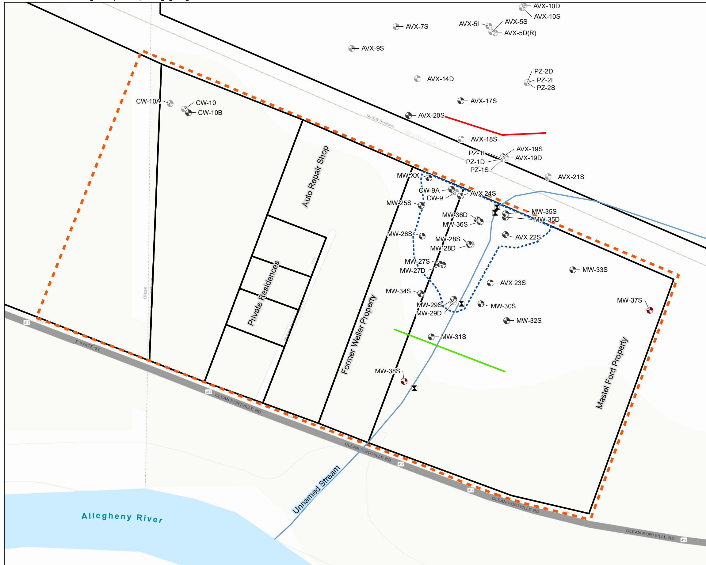
Figure 4-2 Olean Well Field OU4 Alternative 3: Permeable Reactive Barrier with Long-term Monitoring and Institutional Controls Cattaraugus County, NY
