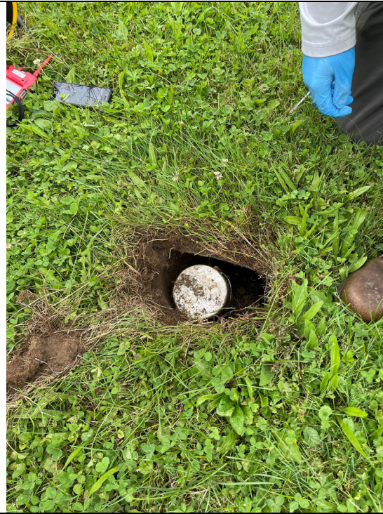
BIA-MW-8 buried underground. Well cover would not come off.
