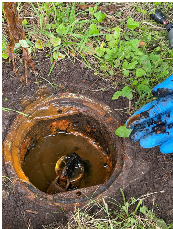
BIA-MW-D2 filled with water. J-plug intact, only well casing full. Dark substance on top of J-plug.
