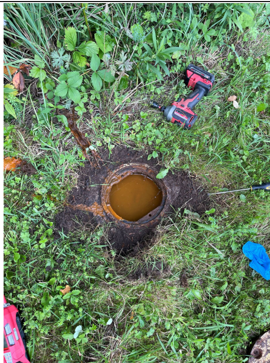
BIA-MW-D2 filled with water. J-plug intact, only well casing full.
