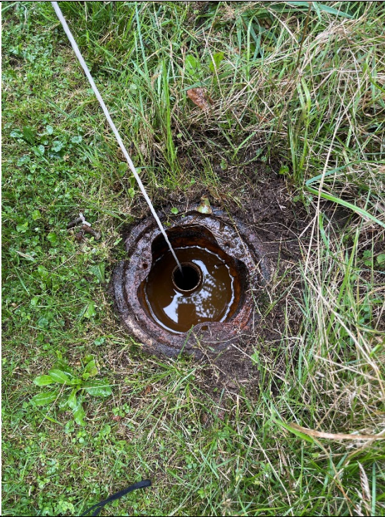
WSA-PZ-45D filled with water. J-plug intact, only well casing full.
