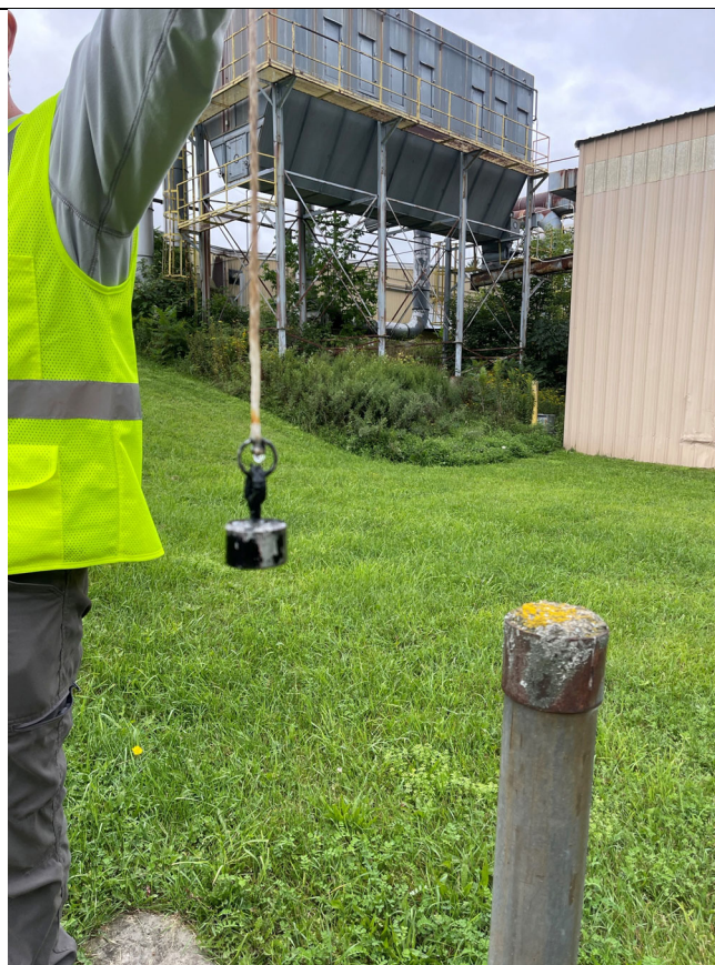
BIA-MW2 has dark substance on end of PDB rope/weight. No distinct odor.
