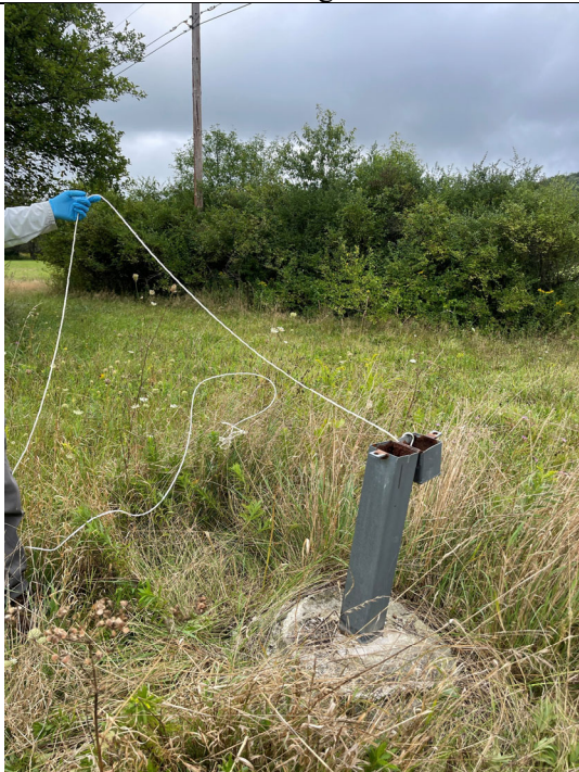
GTA-PZ-25 well casing slightly on an angle
