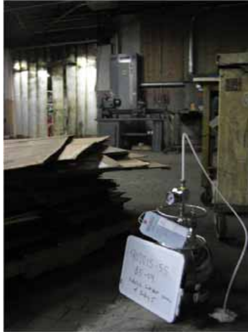
Photo 17: Subslab soil vapor sample 907015-SS-B5-04 in Former Plant 5, looking west.
