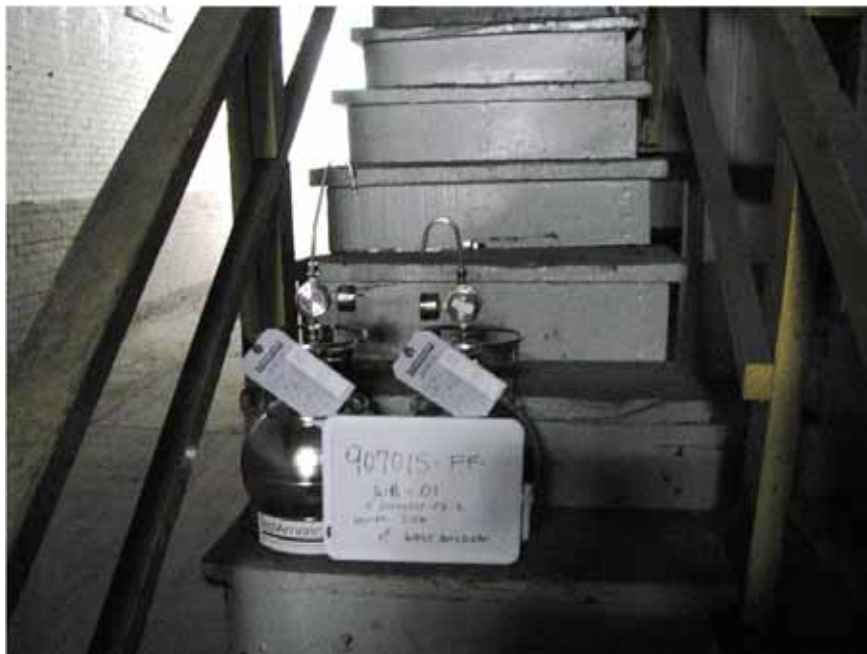
Photo 20: Indoor air sample 907015-FF-WB-01 plus field duplicate in West Building.
