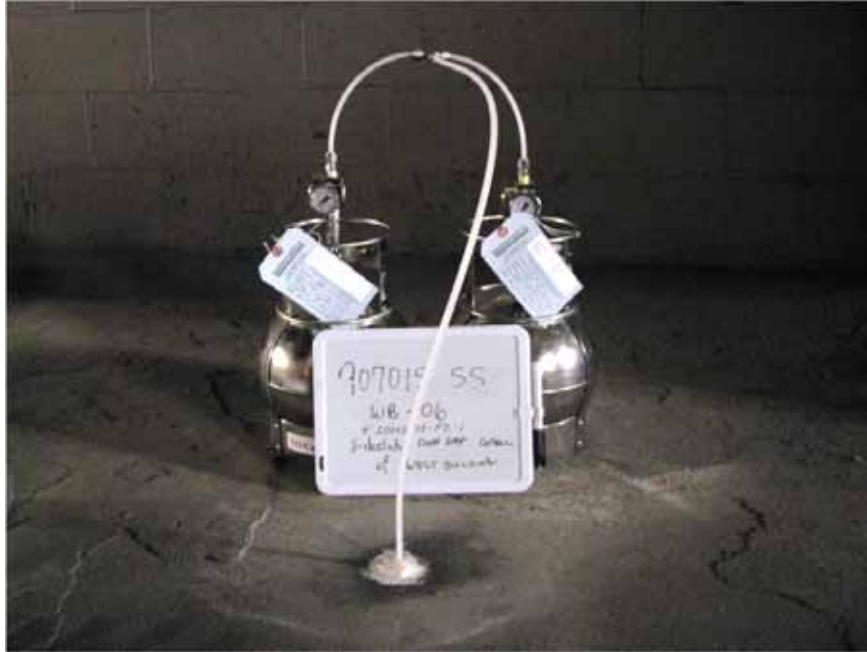
Photo 19: Subslab soil vapor sample 907015-SS-WB-06 plus field duplicate in West Building.
