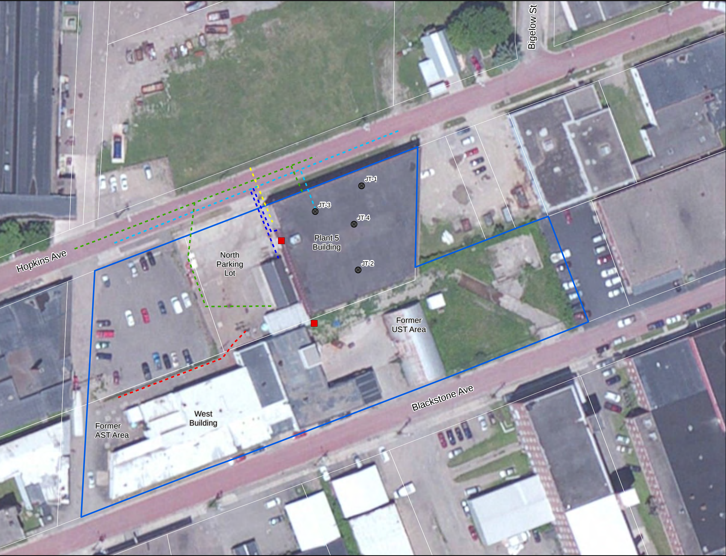
FIGURE 3 Subslab Vapor Probe and Indoor/ Outdoor Pressure Monitoring Locations Vapor Intrusion Investigation and Evaluation Report Jamestown, New York
