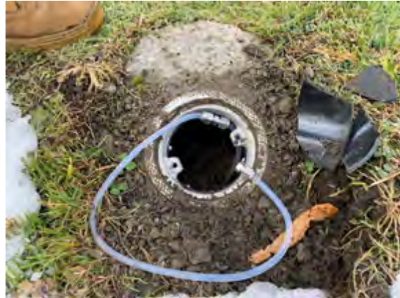
Photograph 18: Broken inner plastic casing: SV-13
