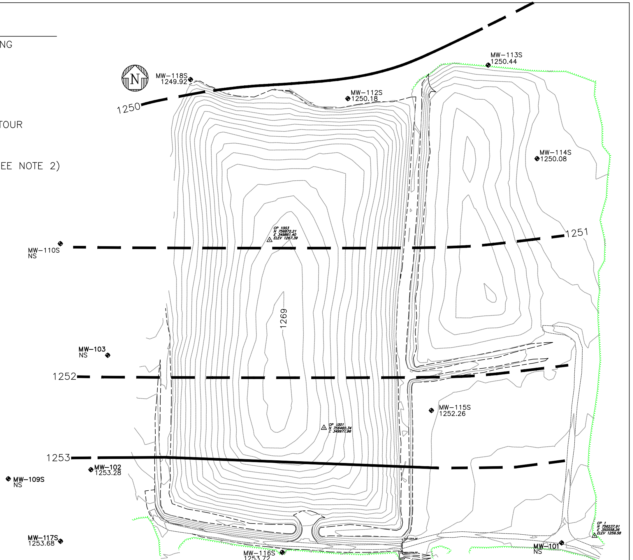
FIGURE 2 GROUNDWATER ELEVATION CONTOURS OF SHALLOW GROUNDWATER WELLS (SEPTEMBER 2019) TOWN OF CARROLL LANDFILL FREWSBURG, NEW YORK
