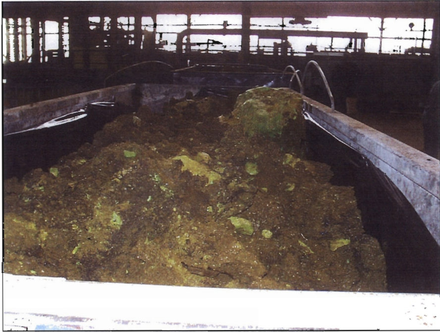
Photo 3. Solidified Kolene residuals (mixed with clay absorbent) in roll-off container
