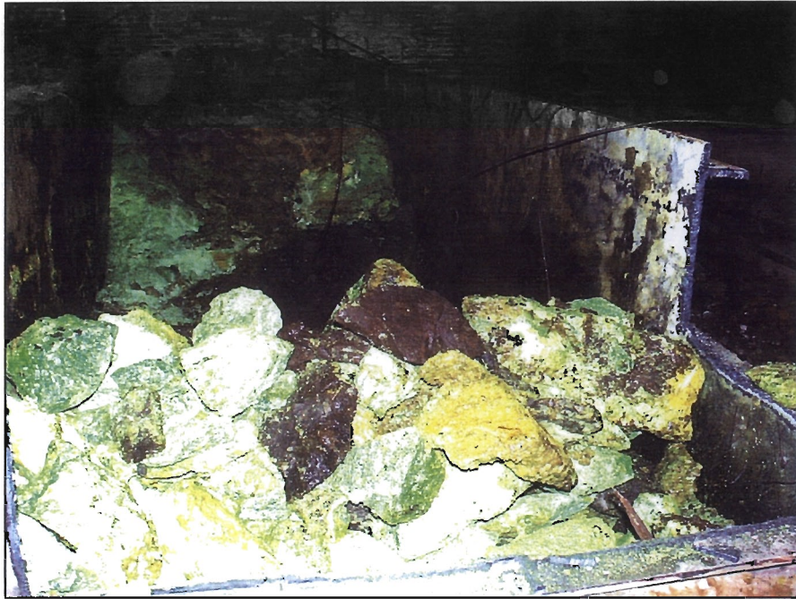
Photo 5. Kolene solids stockpiled in west end of tank
