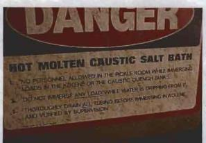
Kolene® is a caustic molten salt pickling bath for the cleaning and descaling of alloy steels. The proprietary salts are heated to a temperature of 850° to 900°F where it attains a liquid, pumpable state.
