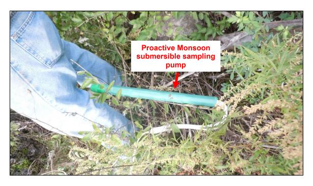
Proactive Monsoon submersible sampling pump used for well purging/sampling.
