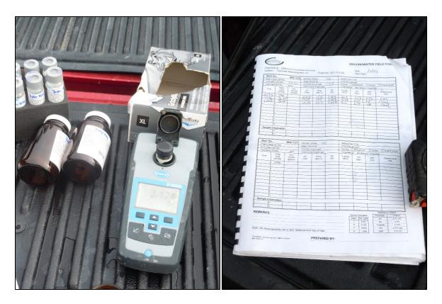
Hach 2100Q turbidimeter (left) and Groundwater Field Form (right).
