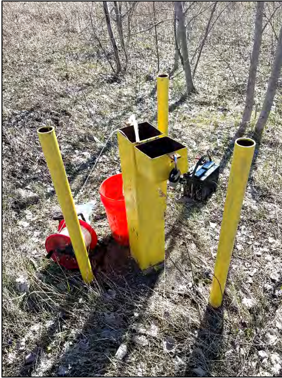
Well MWS-20B (left) and instruments used to record field parameters (right).
