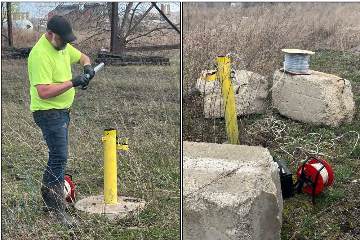
Collecting sample with a bailer at piezometer PZ-9 (left). Installing new dedicated clear PVC tubing in well MWN-72AR (right).
