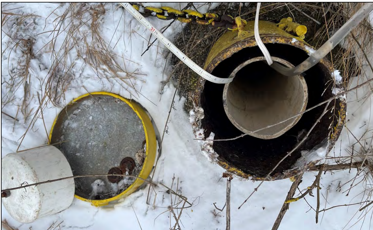
View (from left to right) of water level indicator tape, submersible pump power cord, and dedicated pump tubing in well MW-1D1 during purging/sampling.
