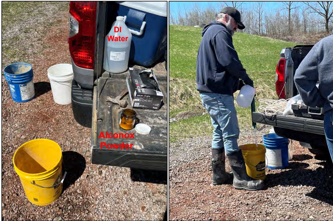
DI Water and Alconox Powder used for decontaminating the non-dedicated submersible pump (left). Tom Behrendt decontaminating the non-dedicated submersible pump over a 5-gallon pail (right).
