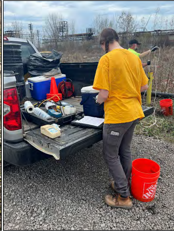
Collecting sample from end of pump tubing at well MWN-72AR (left). Measuring field parameters at well MWN-72AR; in background, Tom is pulling non-dedicated submersible pump from MWN-72AR (right).
