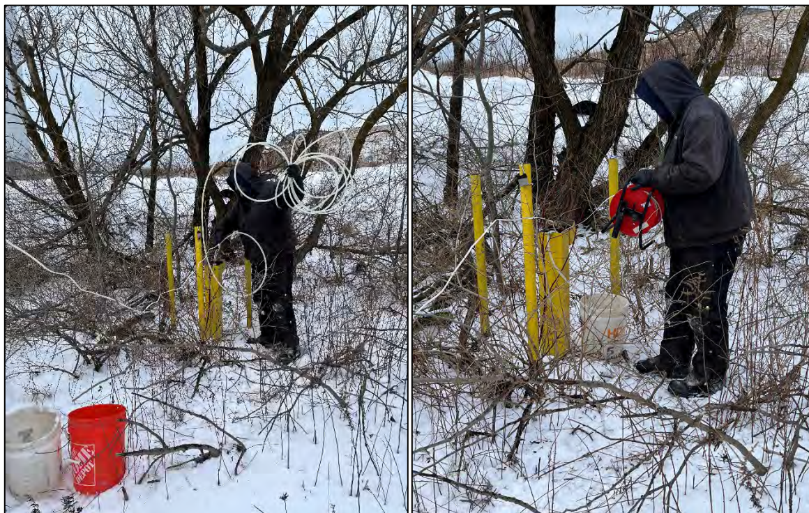
Installing submersible pump and tubing into well MW-1D7 (left). Measuring depth to water and bottom in MW-1D7 (right).
