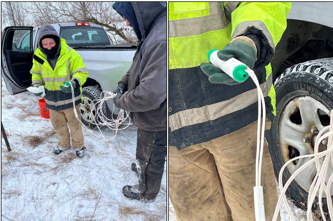
12-volt electric submersible sampling pump.
