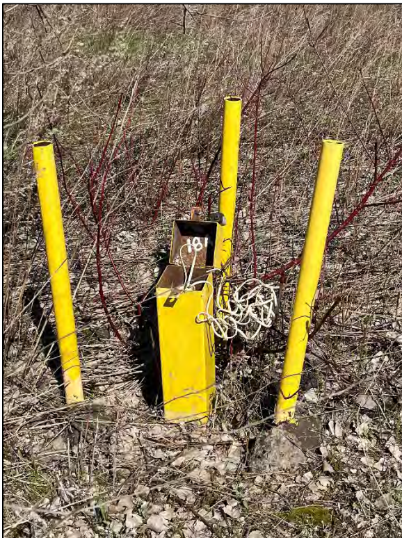
Well MWS-18A (left; showing power cord from dedicated submersible pump at wellhead) and well MWS-18C (right; no dedicated submersible pump).
