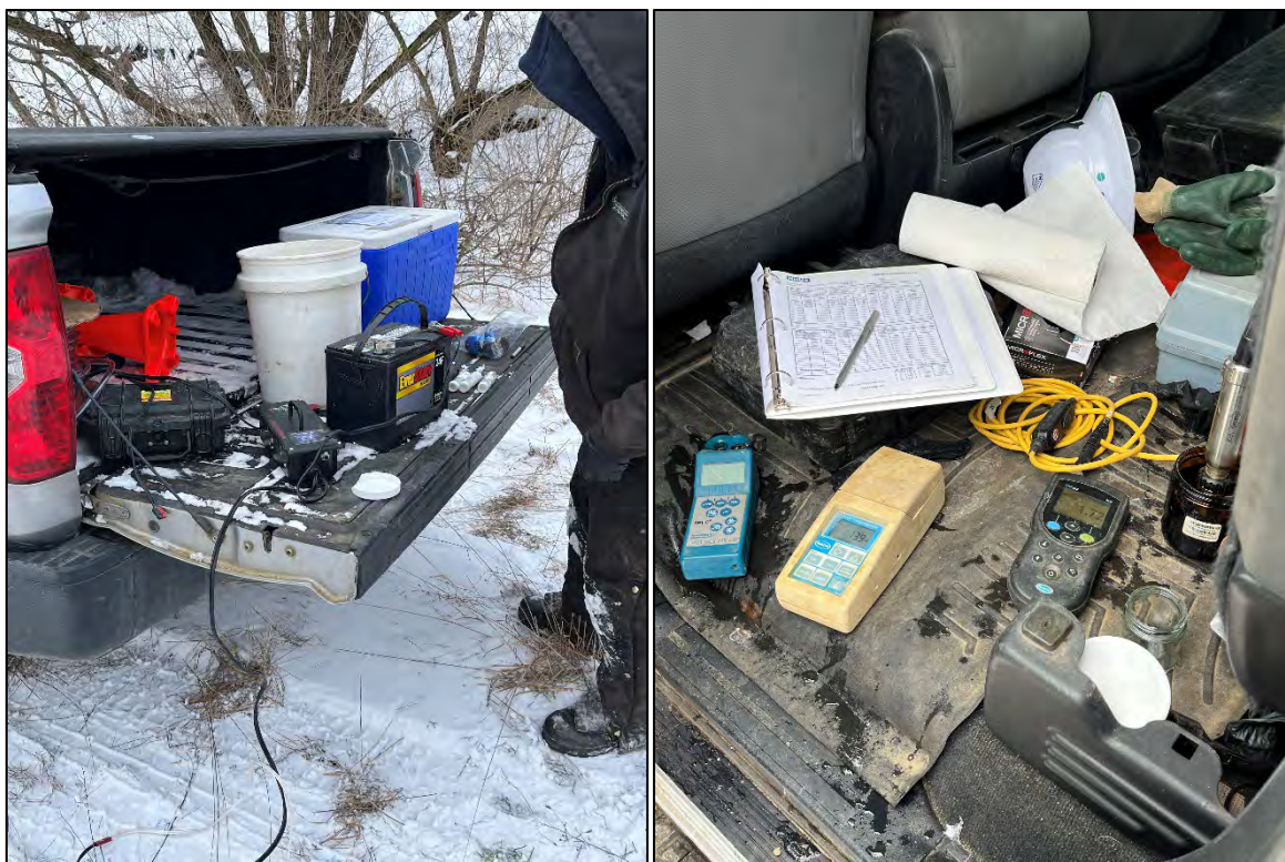
View of submersible pump 12-volt deep cycle battery and low-flow controller box (left). View of instruments used to record field parameters (right).
