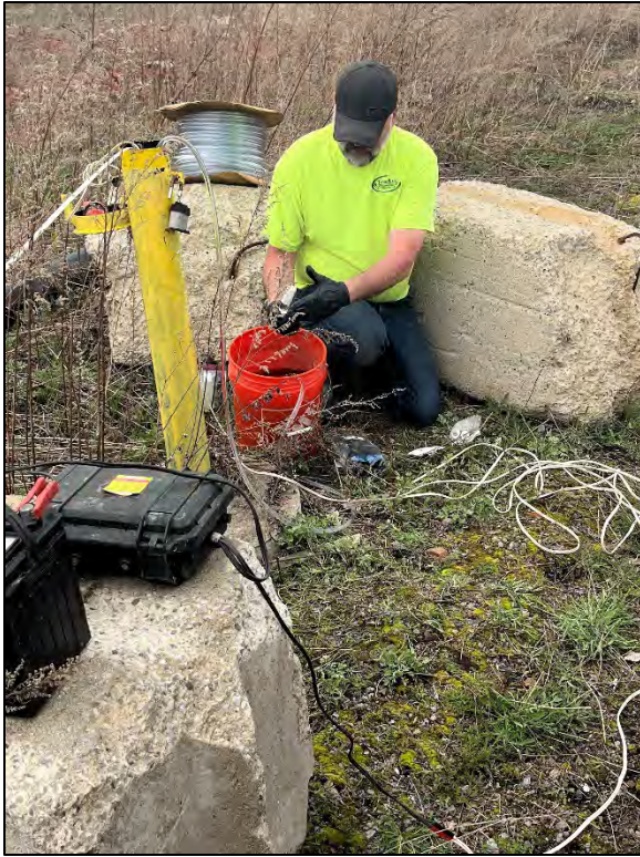
Collecting sample from end of pump tubing at well MWN-72AR (left). Measuring field parameters at well MWN-72AR; in background, Tom is pulling non-dedicated submersible pump from MWN-72AR (right).
