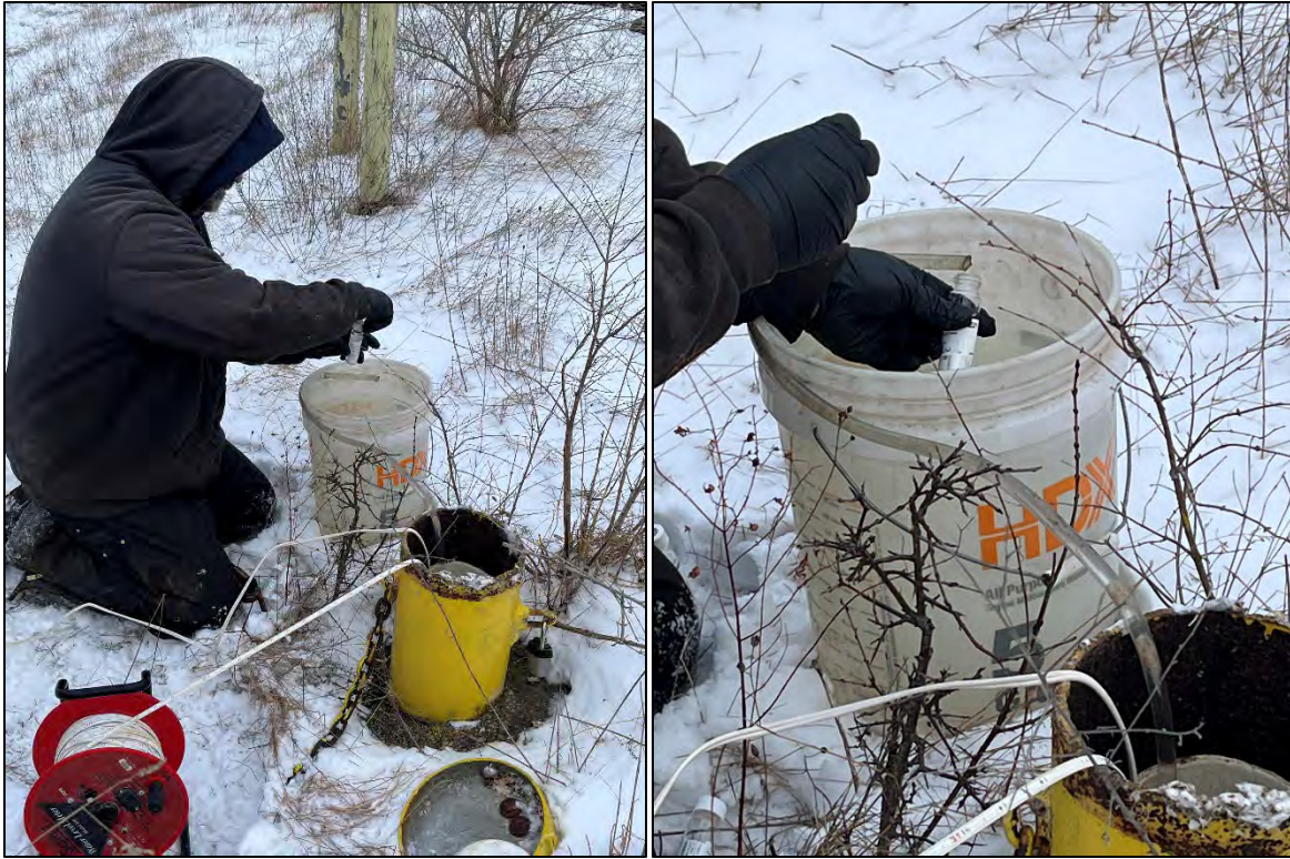
Filling VOC sample vial from end of pump tubing at well MW-1D1.
