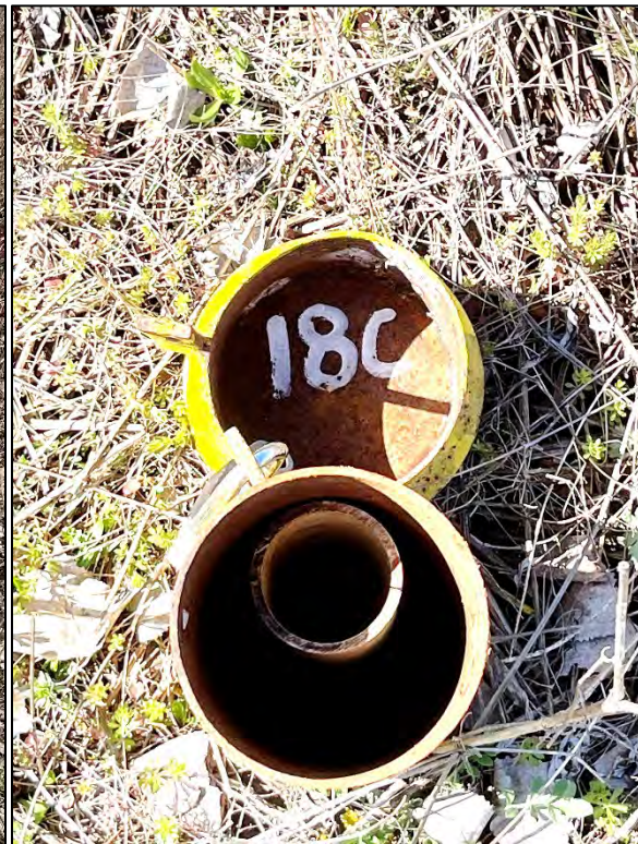
Well MWS-18A (left; showing power cord from dedicated submersible pump at wellhead) and well MWS-18C (right; no dedicated submersible pump).
