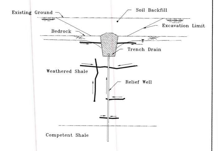
Groundwater Extraction System Detail
