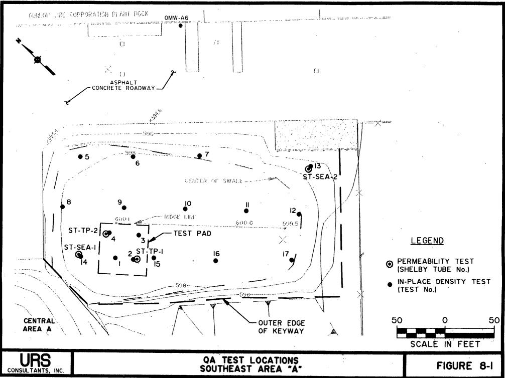
The QA tests of the test pad produced acceptable density results. Shelby tube samples for permeability testing were obtained from the entire 18-inch LPS depth. Two (2) samples were taken from each tube; one from the bottom 6 inches, and one from the middle 6 inches. All four samples were tested, and all showed permeability results less than the specified  $1.0 \times 10^{-7}$  cm/sec.
